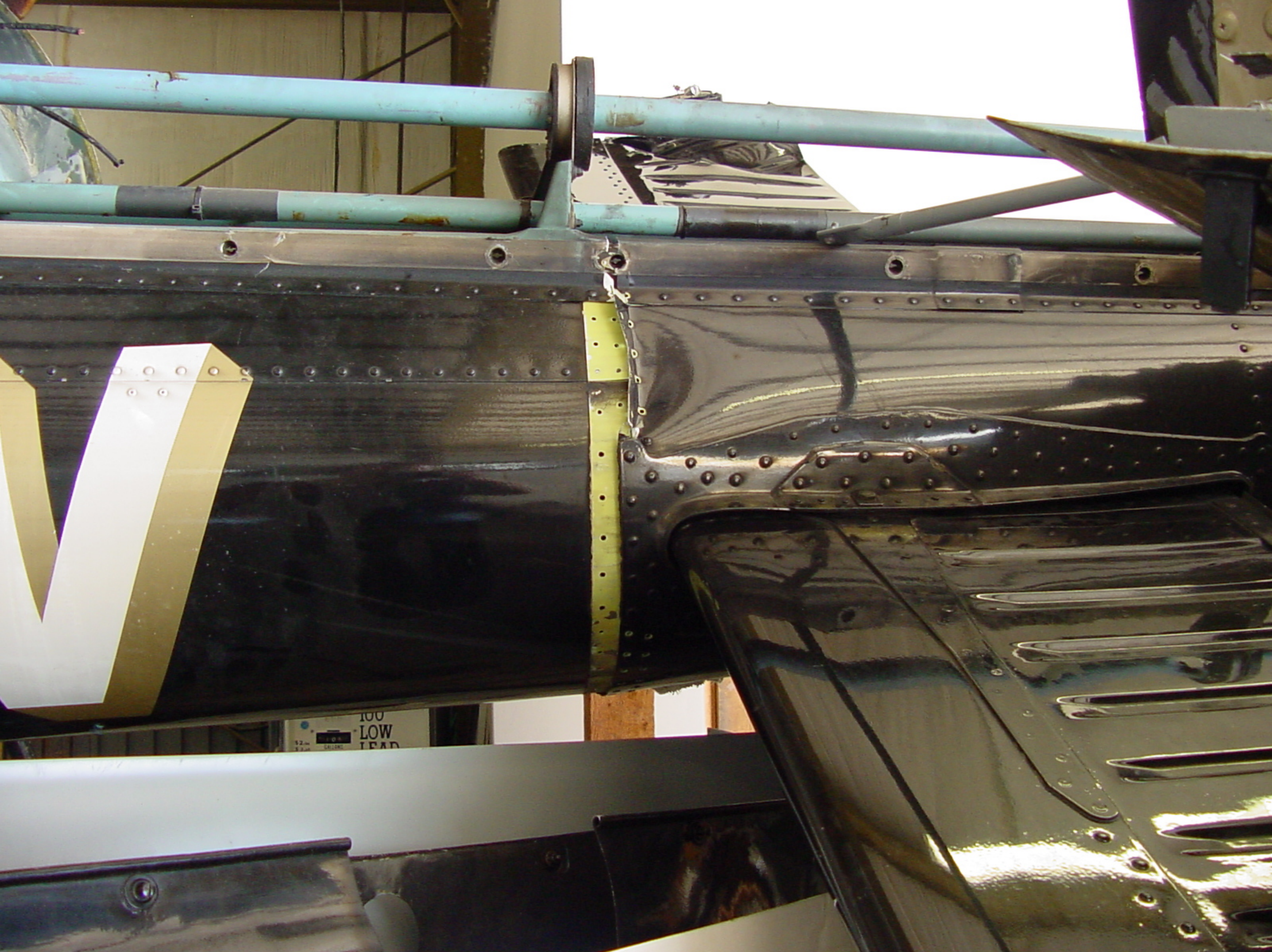
Photo 32. Side View of Scuff Sleeve (Eurocopter Photo)
