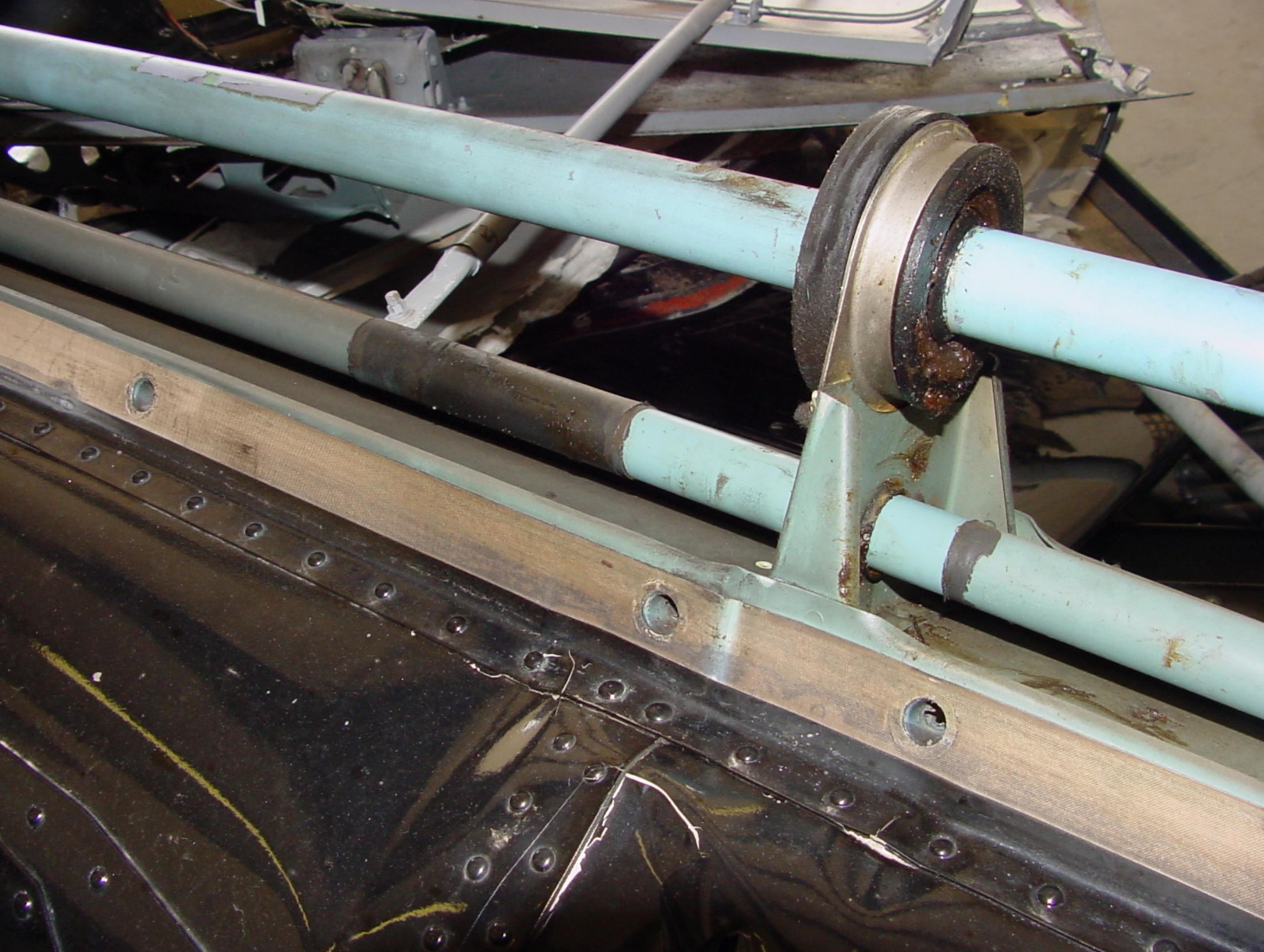
Photo 31. Scuff Sleeve Positioned Aft of Bracket. Note Pro Seal Forward of the Bracket (Eurocopter Photo)
