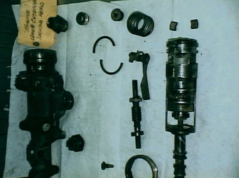
Photo 31. No. 1 engine reverser hydraulic actuator upper outboard locking head.
