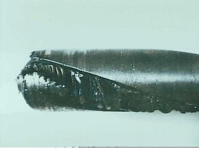
Photo 30. Example of a delta drill used without coolant. A heavy accumulation of chips accured during the testing.
