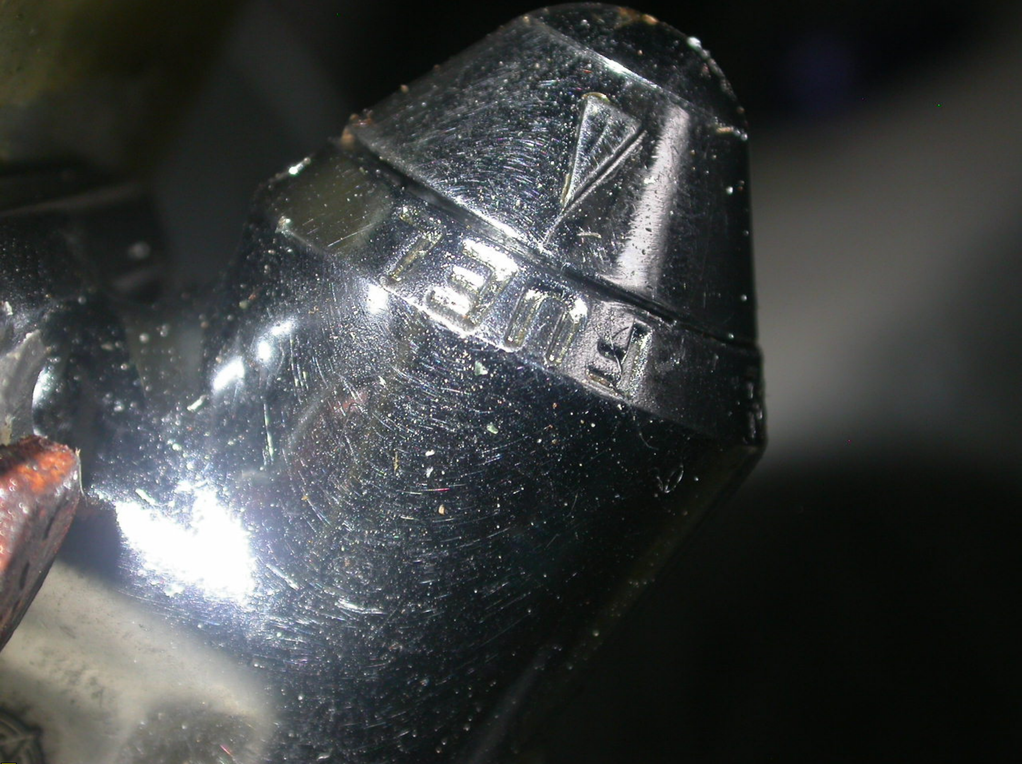
Photo 3. Fuel selector, showing it positioned in the FUEL (on) position.
