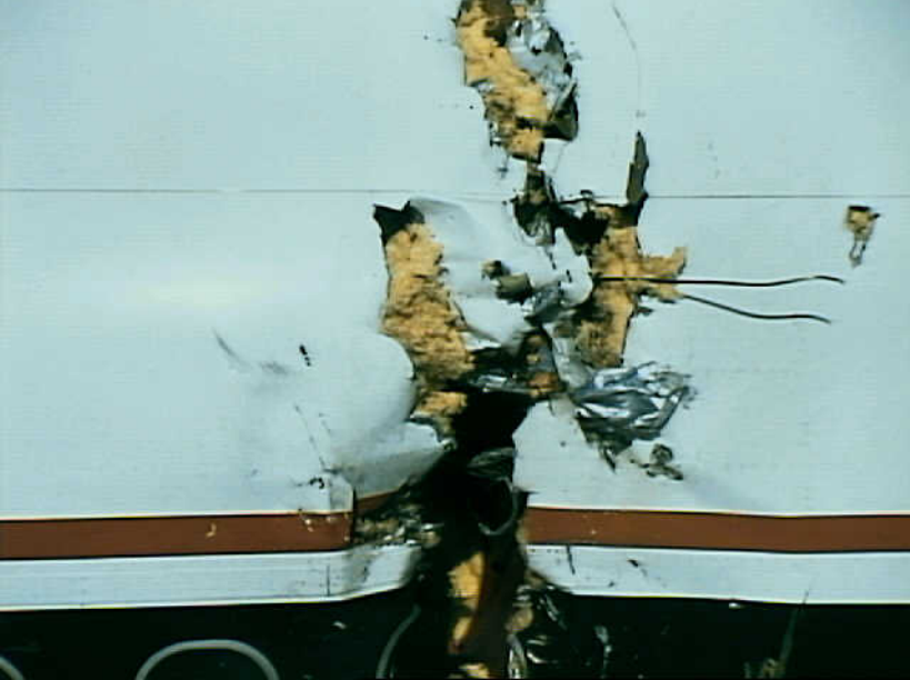
Photo 3. Left fuselage penetration damage.
