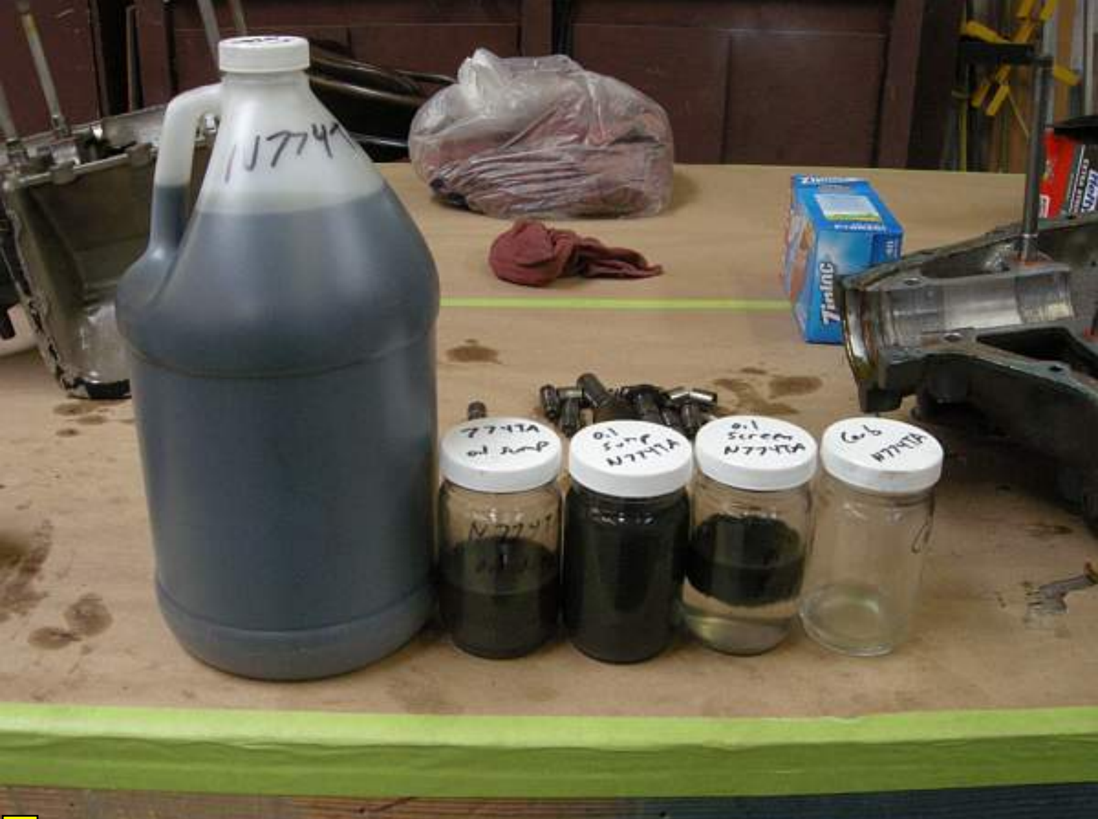
Photo 3 - Recovered Oil from Engine
