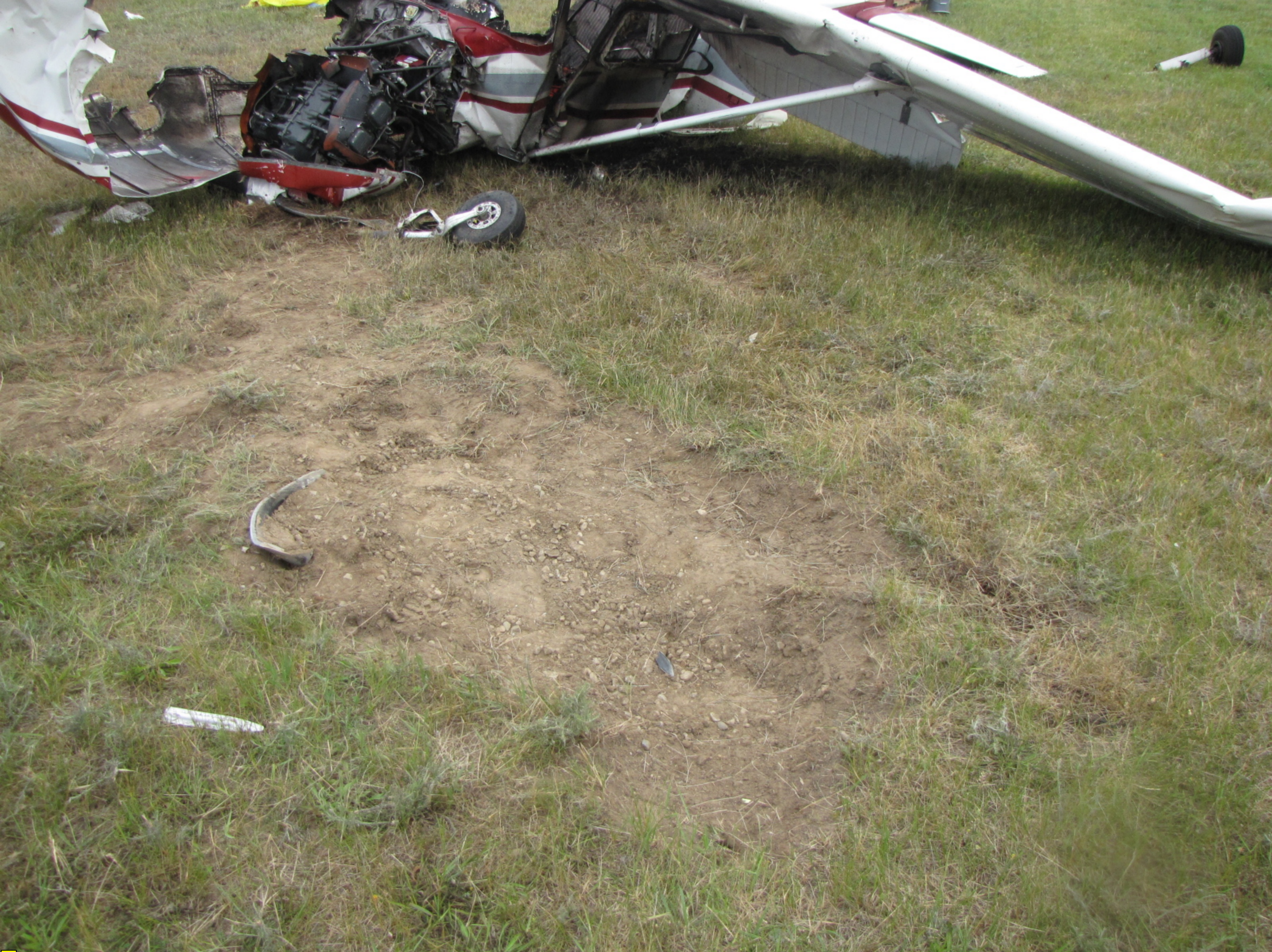
Photo 3 - Ground scar and crater containing propeller blade.
