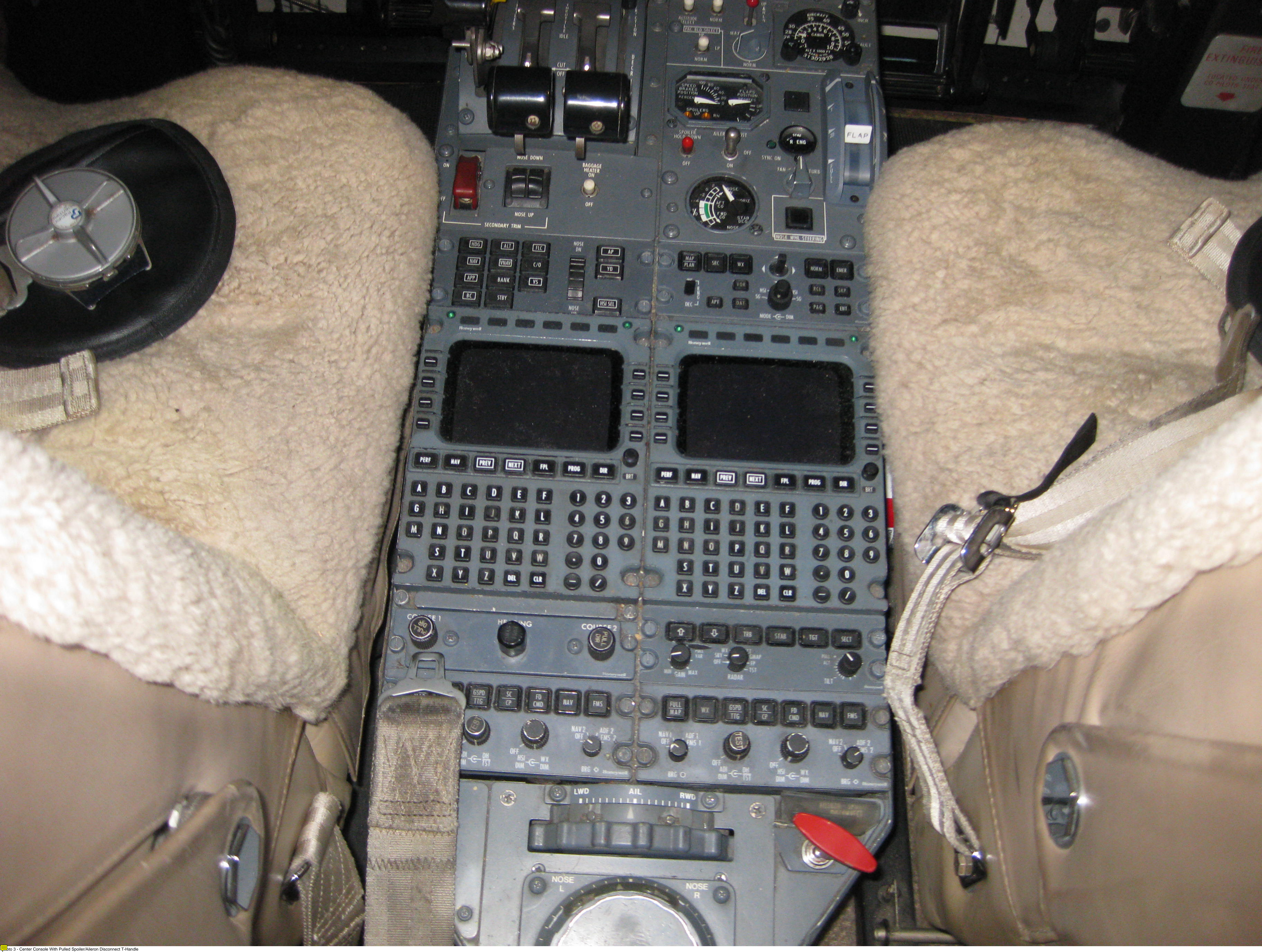
Photo 3 - Center Console With Pulled Spoiler/Aileron Disconnect T-Handle
