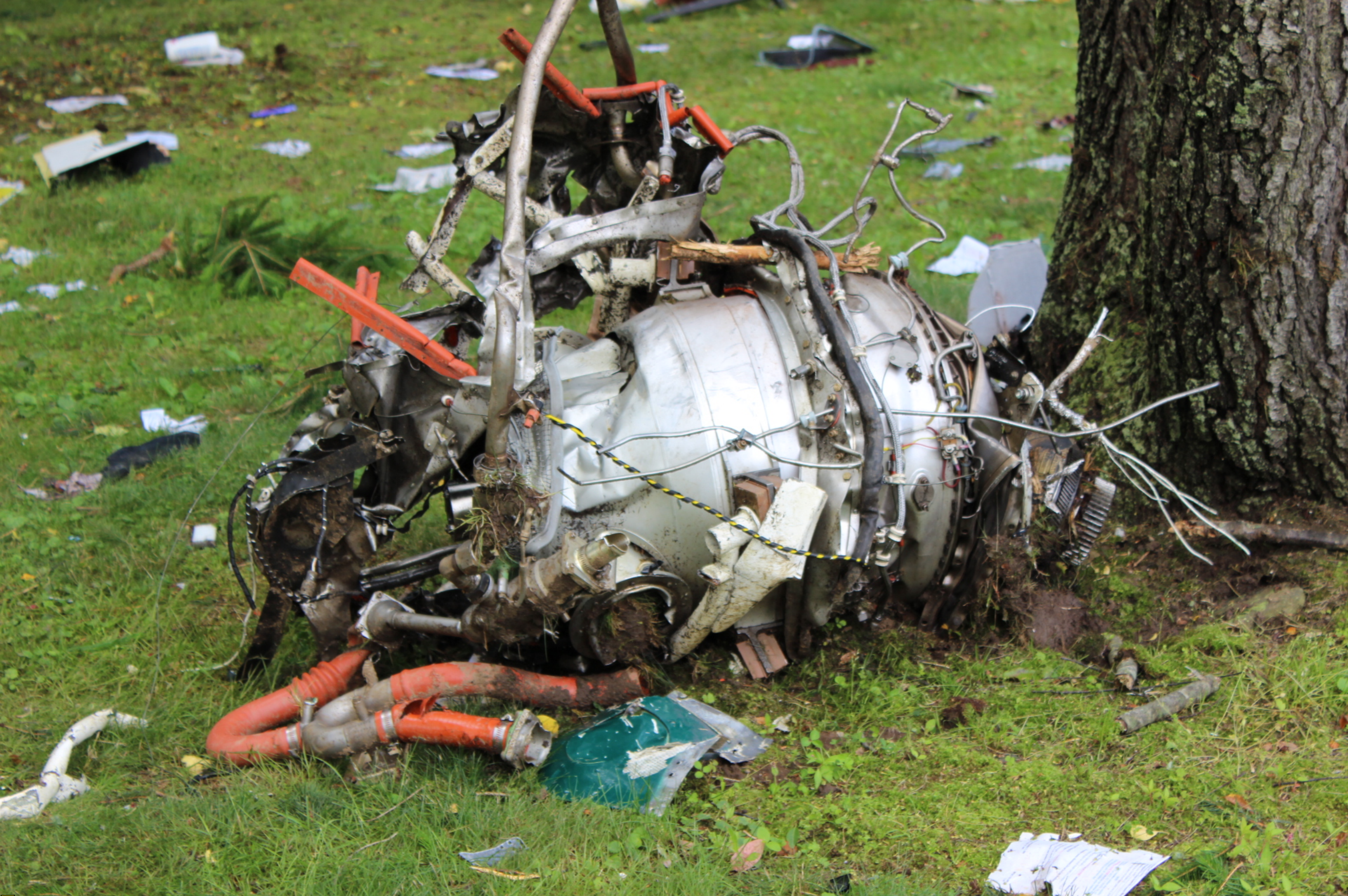
Photo 3 - View of Engine as Found (PWC)
