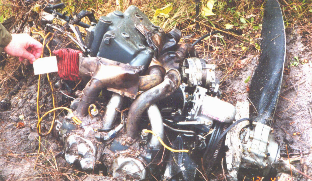
Photo 3: View of the separated left engine with attached propeller hub and 1 propeller blade from N3038N
