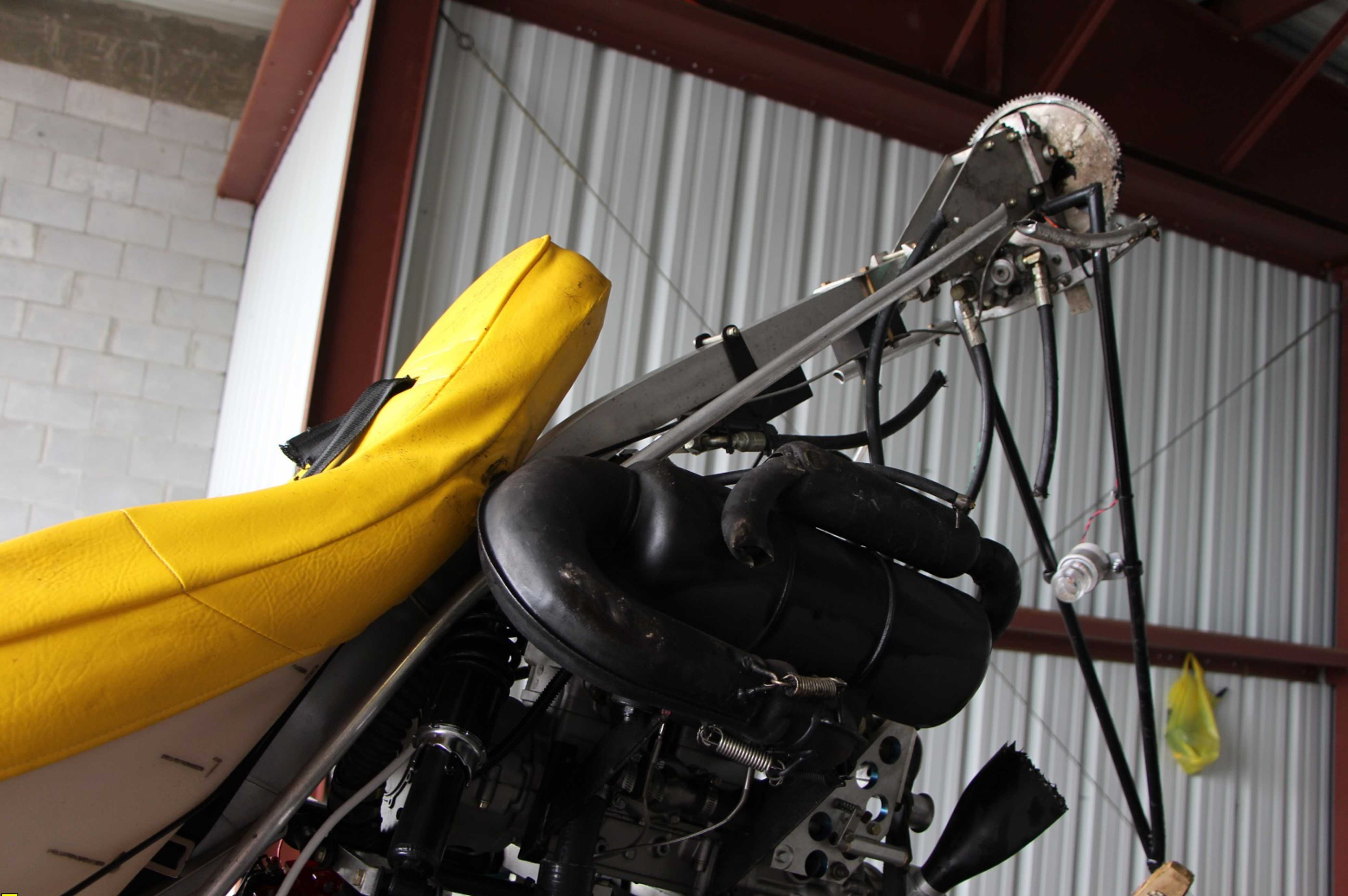
Photo4: Picture of the Bent Mast.
