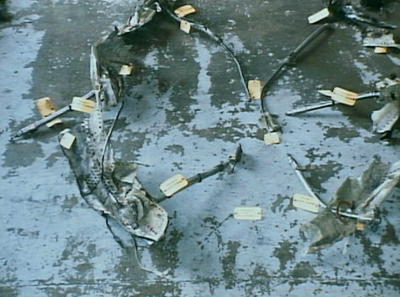
Photo 29. No. 2 engine reverser hydraulic actuators and TB/FW fragments
