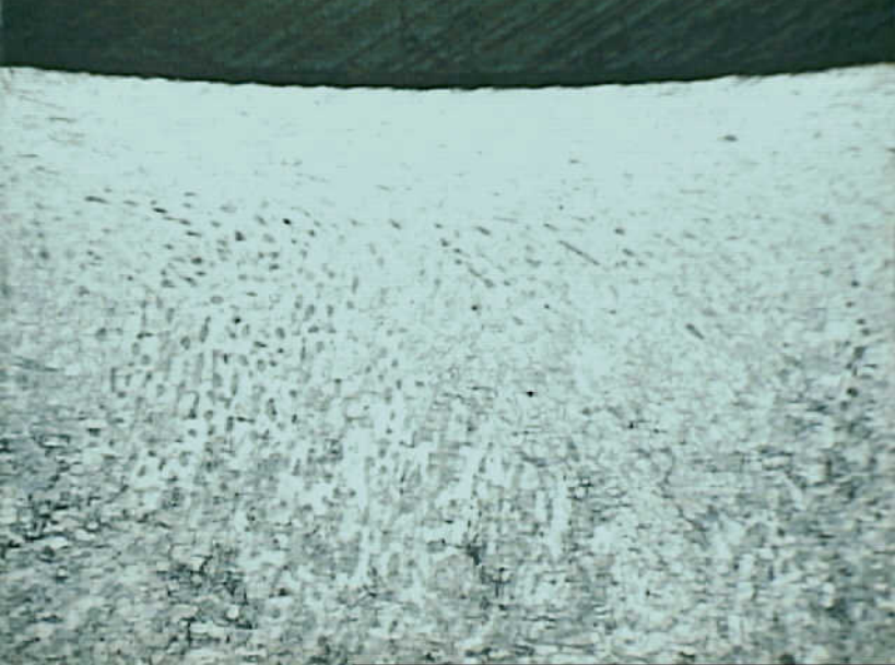
Photo 29. A close up of photo 28. Microstructure of hole #52 showing deformed and overheated material to a depth of 0.6 - 0.7 mm (0.024-0.028 inch). Mag 64X.
