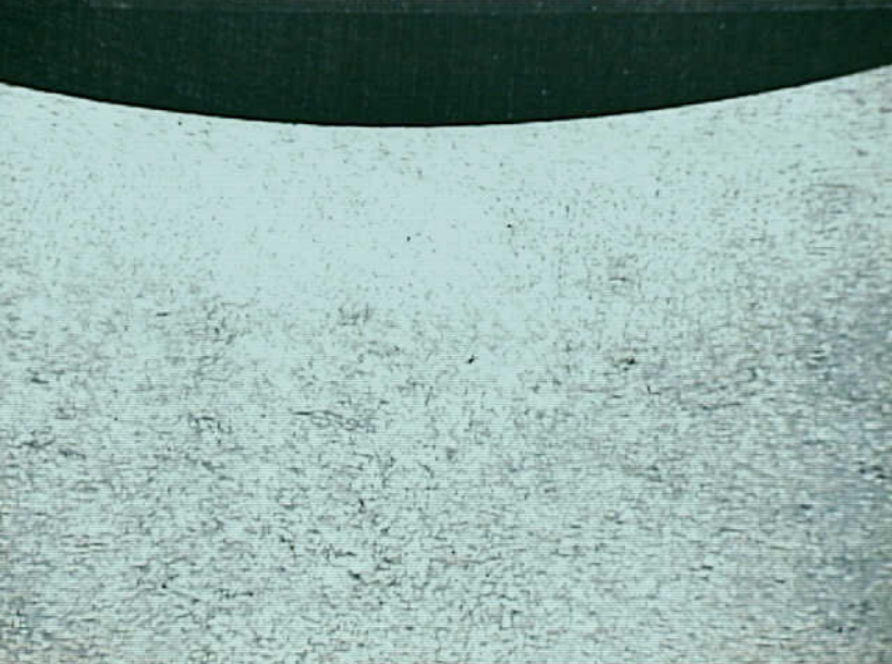
Photo 28. Microstructure of hole #52 showing deformed and overheated material. Mag. 32X.
