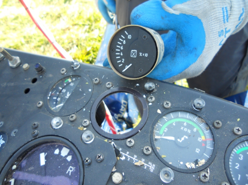
Photo 28: View of fuel quantity gauge
