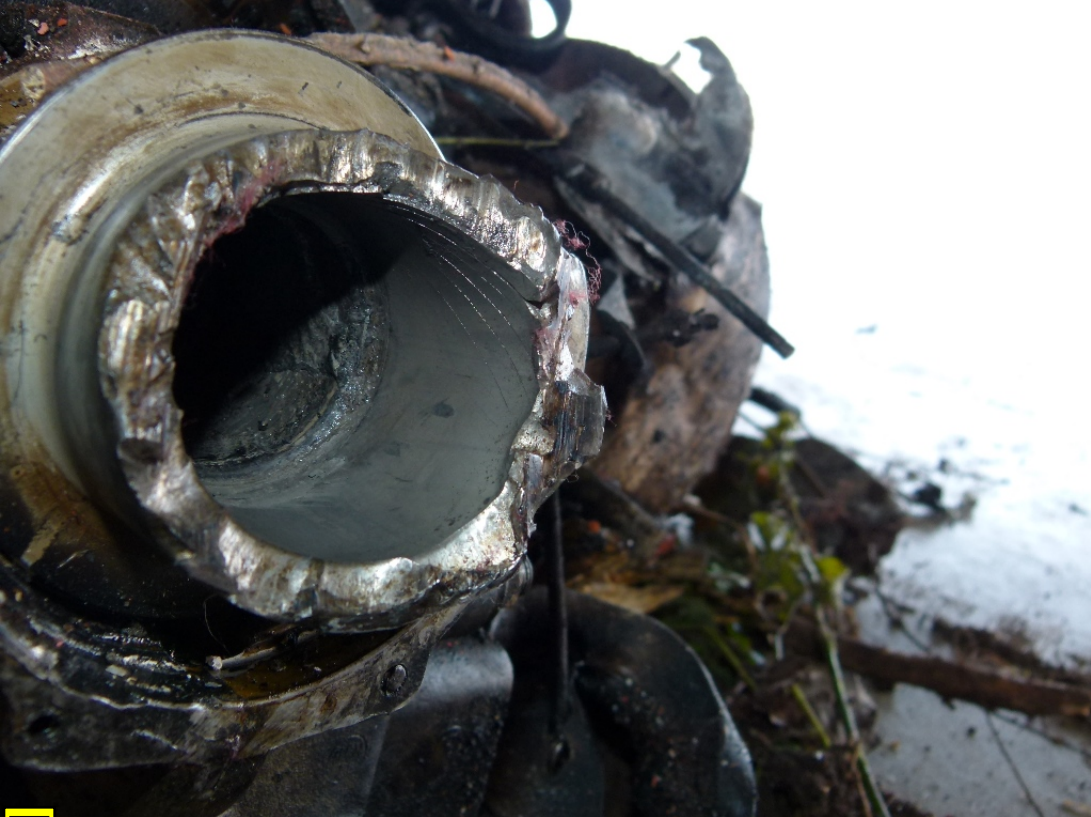
to 26. Another view of the fractured crankshaft.
