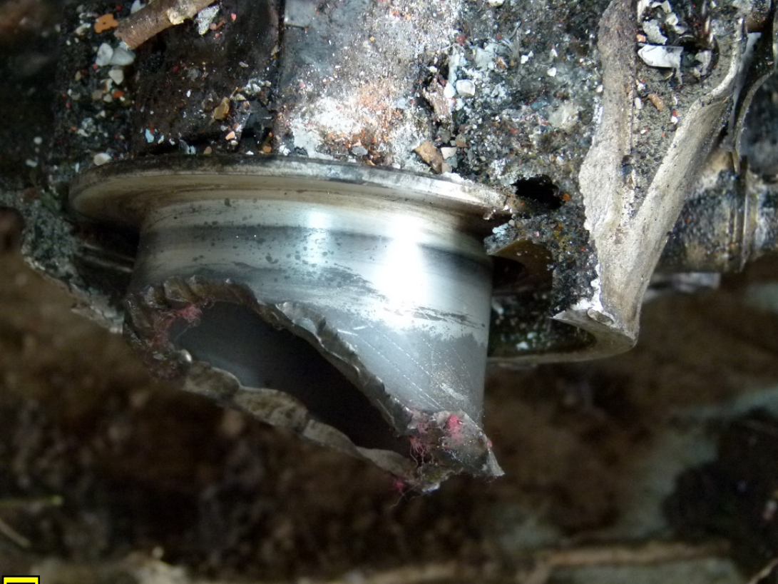
Photo to 25. View of fractured crankshaft.
