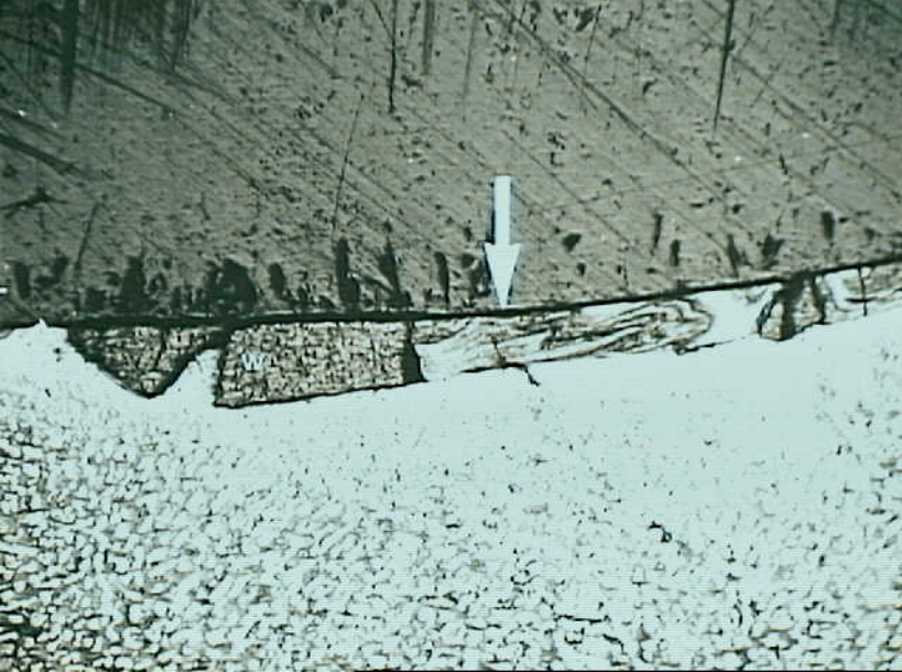
Photo 25. A close up on the indication area in hole #57 in previous photo. During the drill breakdown particles on tungsten (W) have been pressed into the ID.
