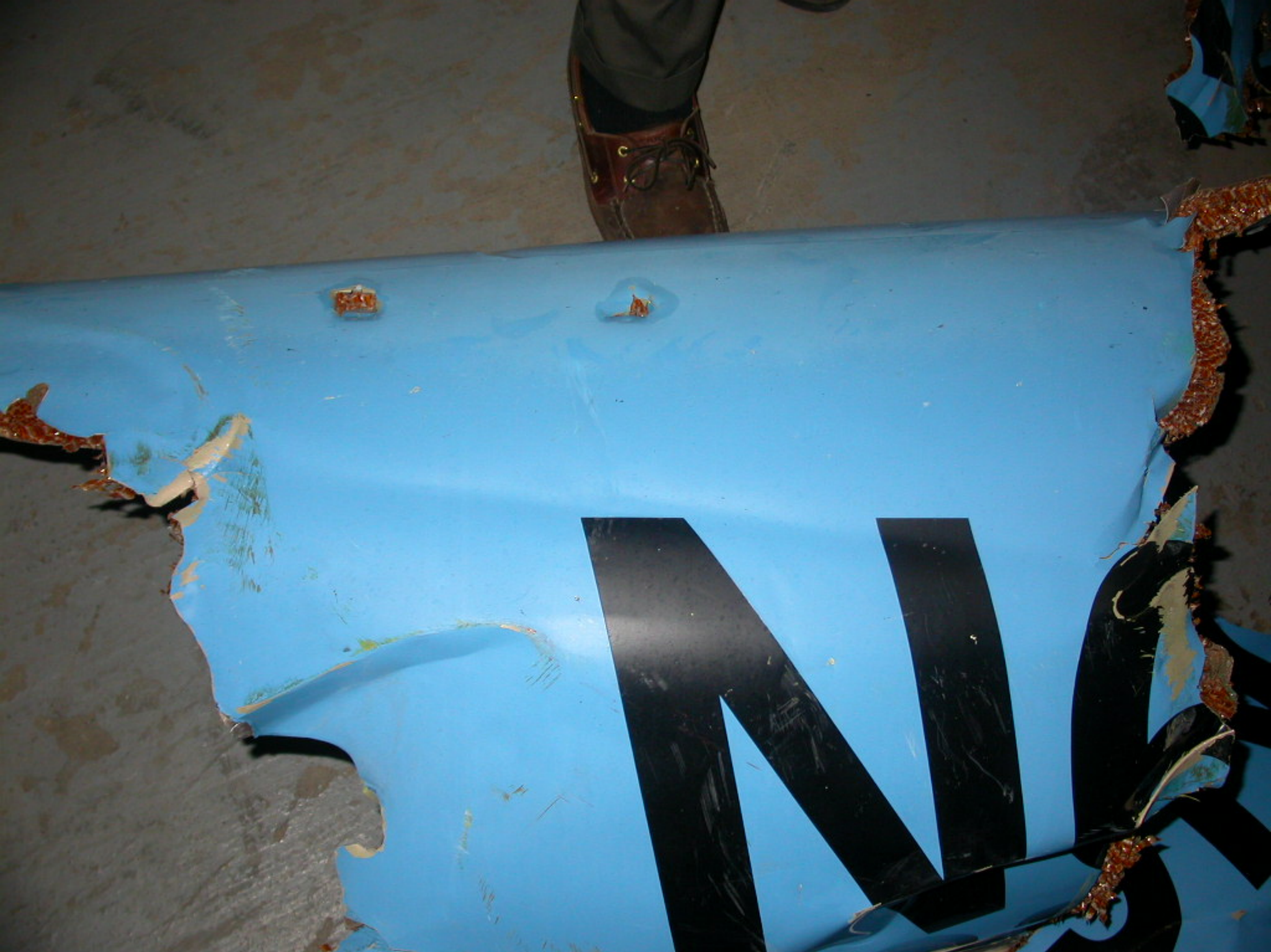
Photo 24. Puncture Holes on Tail Cone Structure
