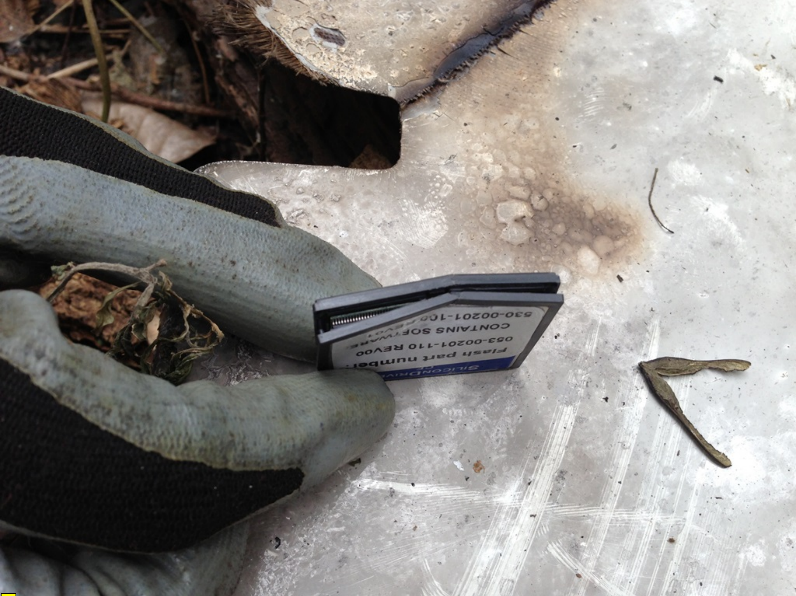
Photo 23. View of damaged MFD memory card.
