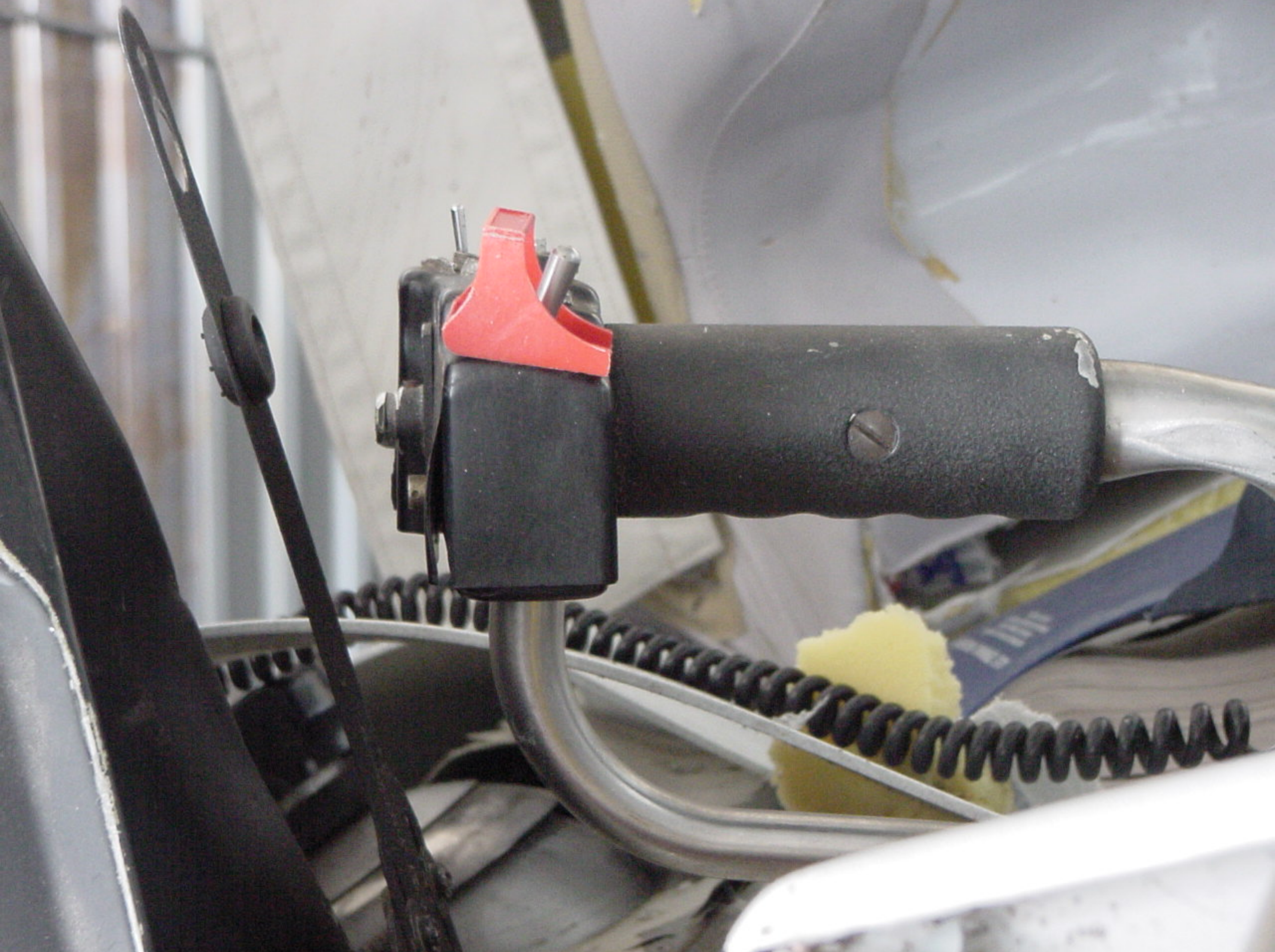
Photo 23. Hydraulic Switch on Collective
