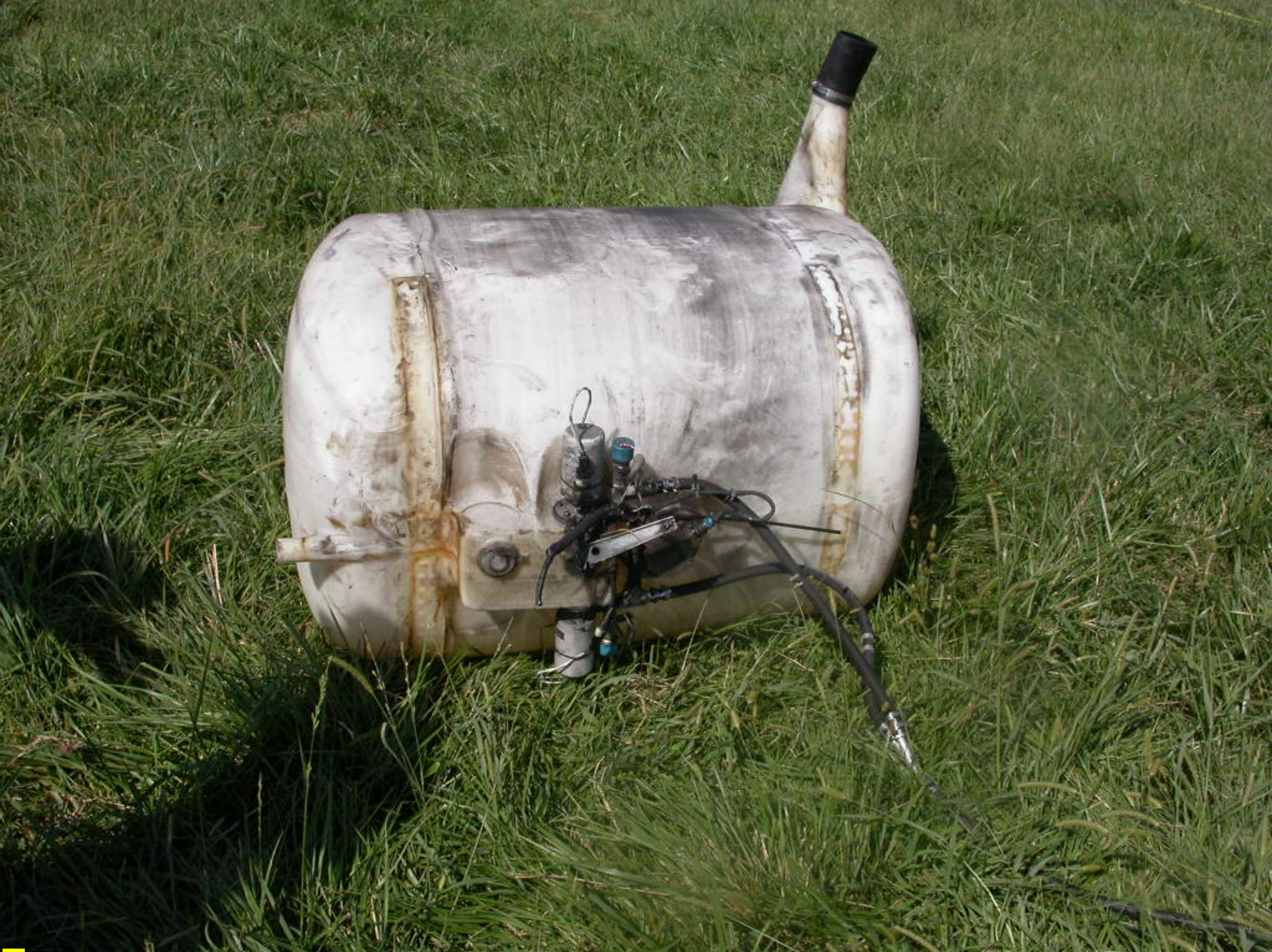
Photo 23: View of the intact fuel tank removed from the main wreckage
