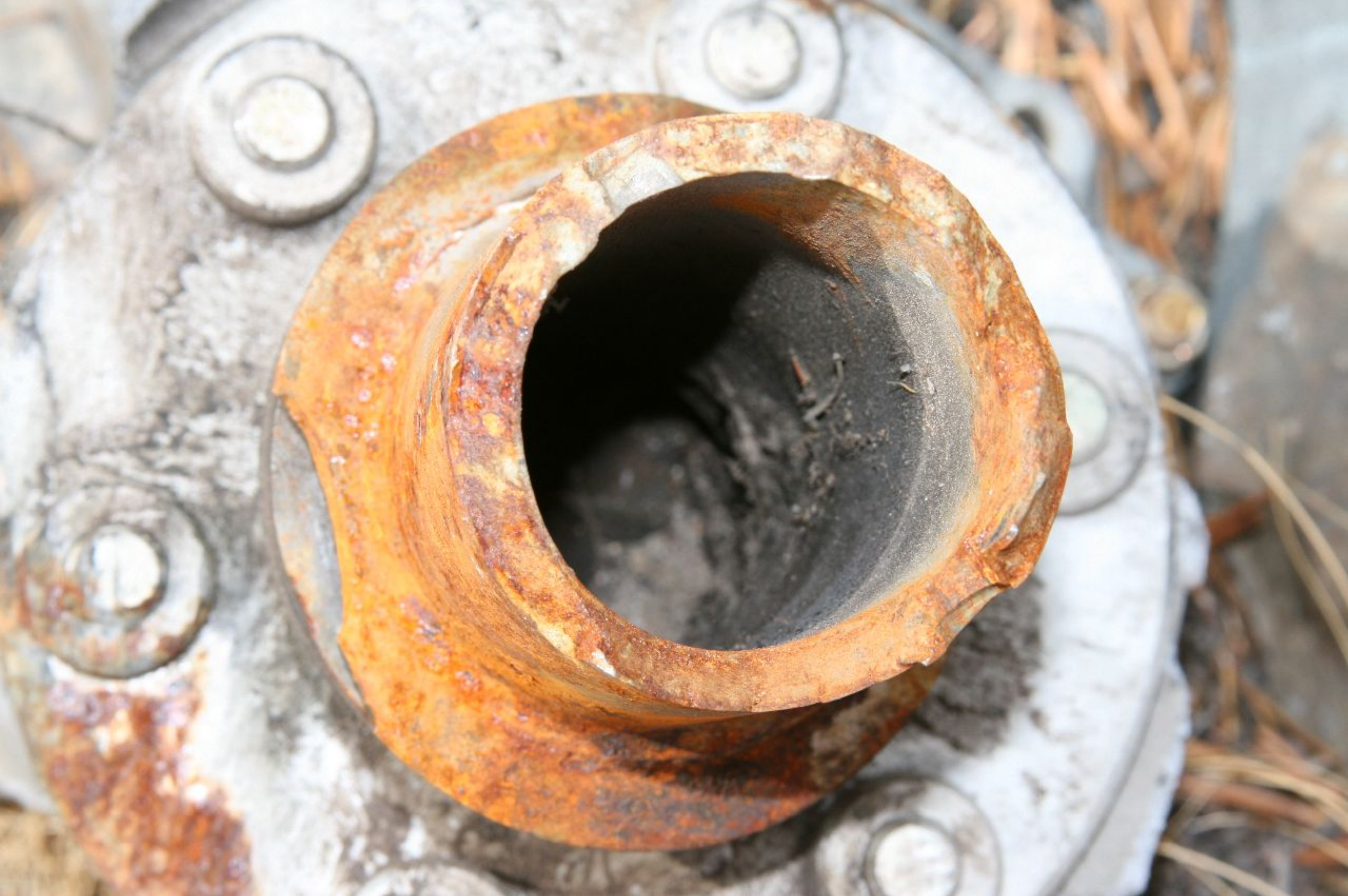
Photo 22. Crankshaft fracture surface.
