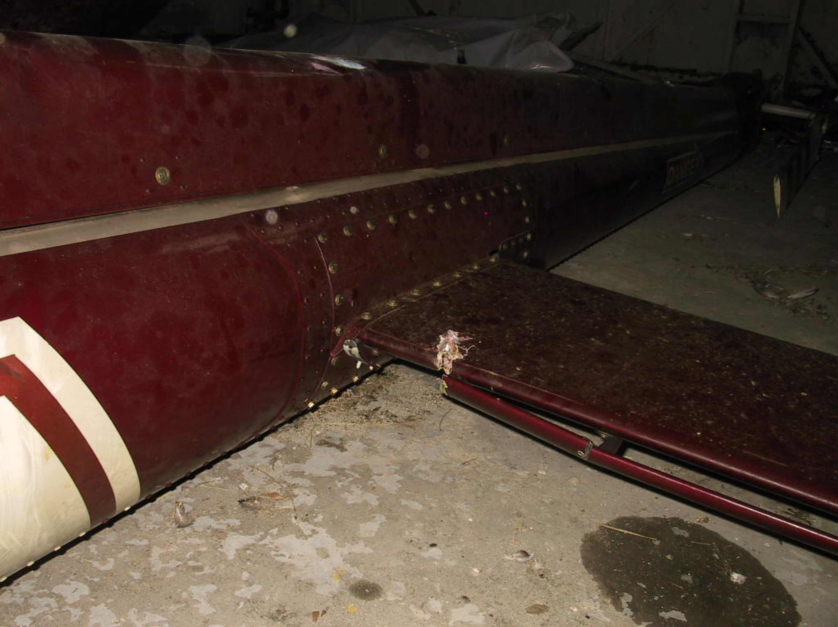
Photo 22. Slash in Leading Edge of Left Horizontal Stabilizer (Bell Photo)
