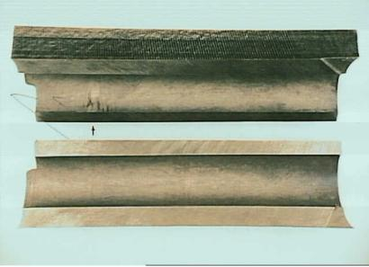
Photo 22. Hole #57 drilled with increased cutting data with HM to breakdown. The hole has also been fine bored and honed. BEA shows a white-grey indication in the drill breakdown area.
