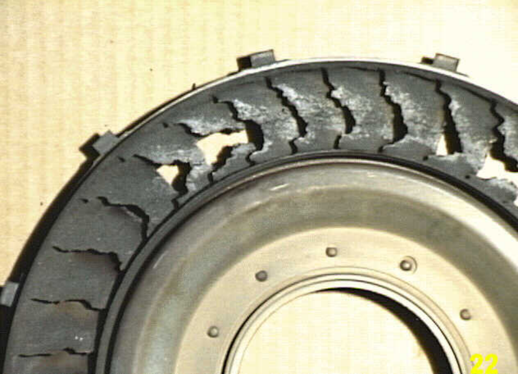
Photo 22 Right Engine and Propeller-Low pressure turbine vane ring, downstream side
