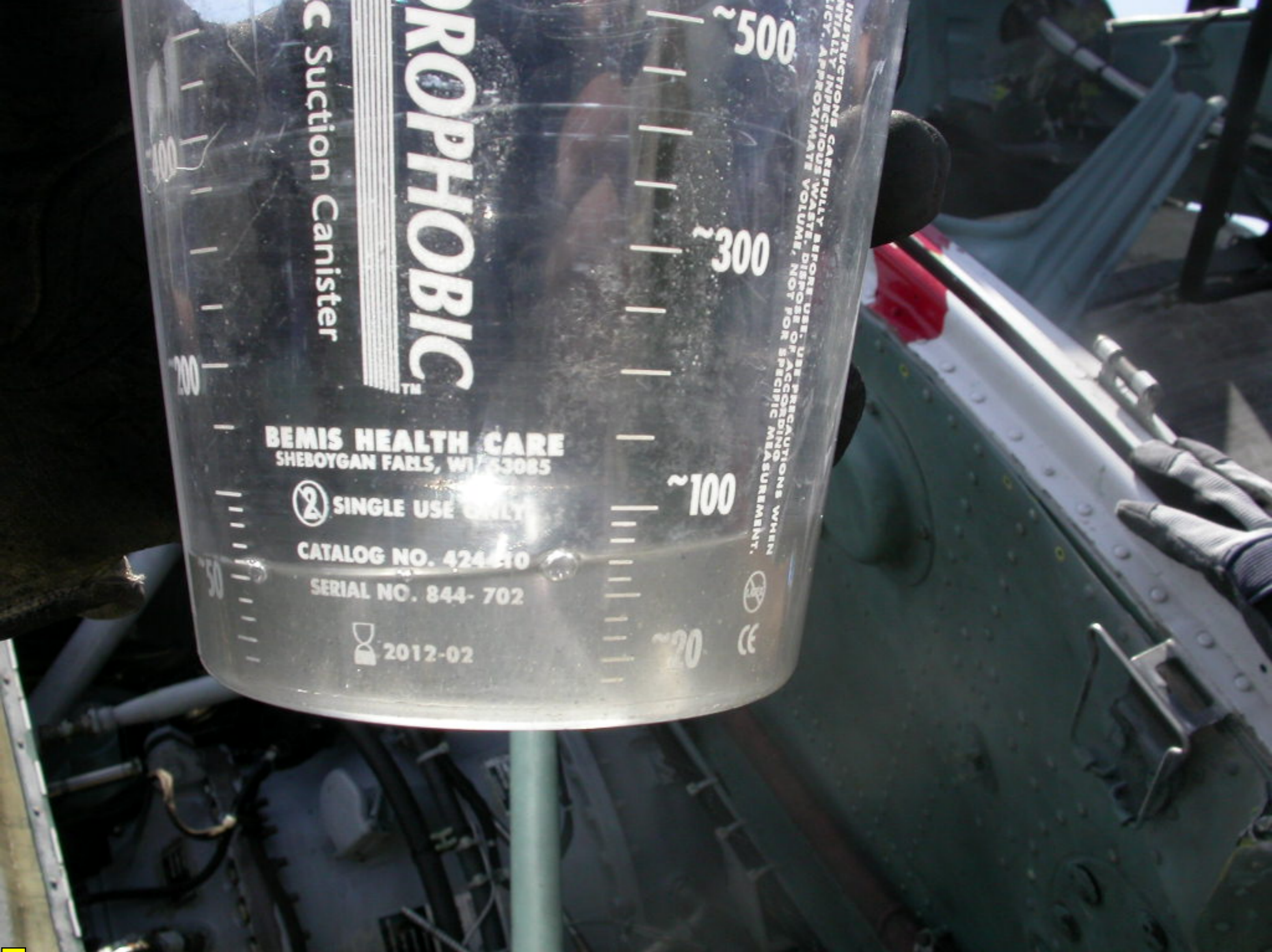
Photo 22: View of the fuel found in the fuel lines
