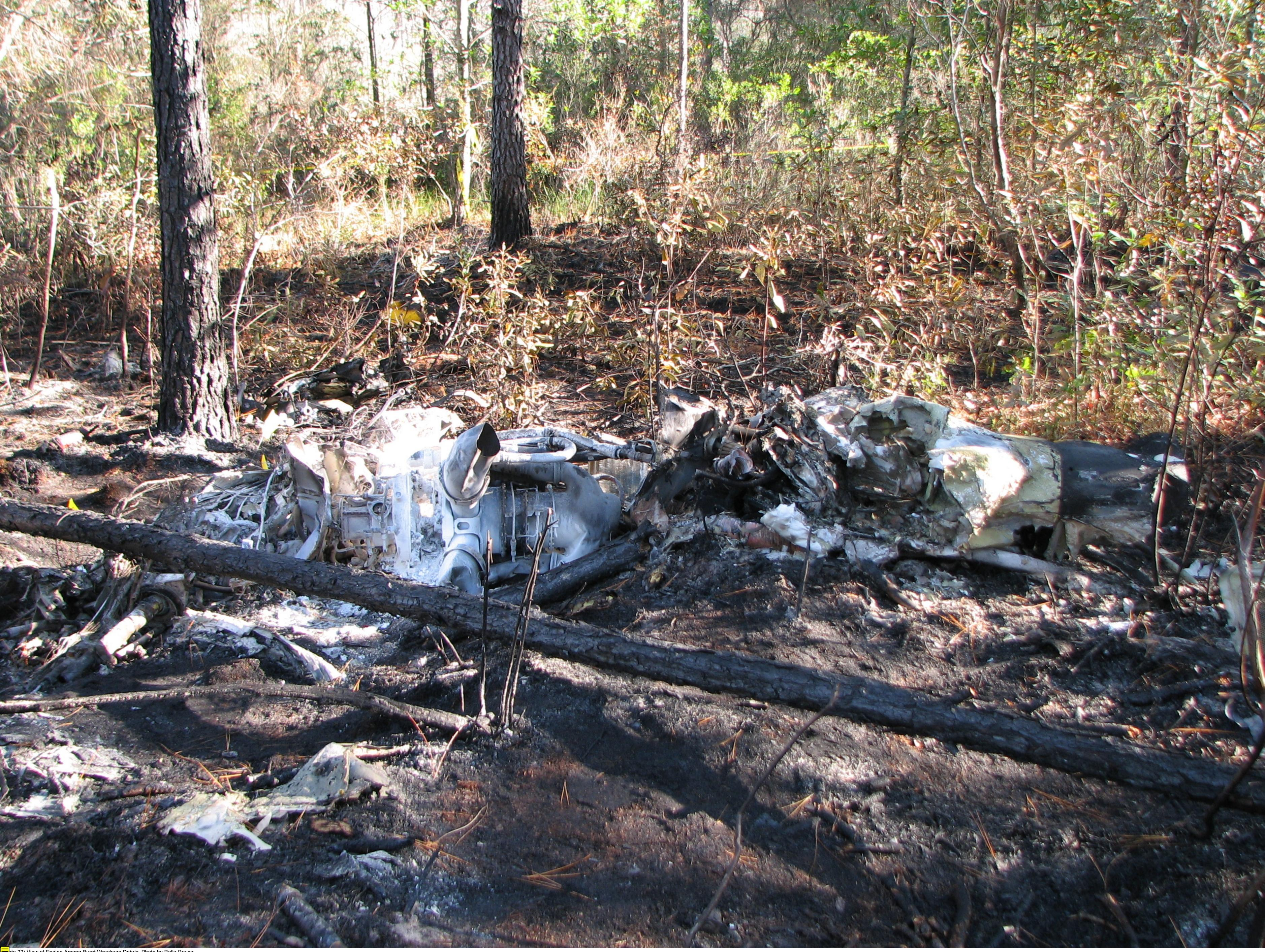
bto 22) View of Engine Among Burnt Wreckage Debris. Photo by Rolls-Royce.
