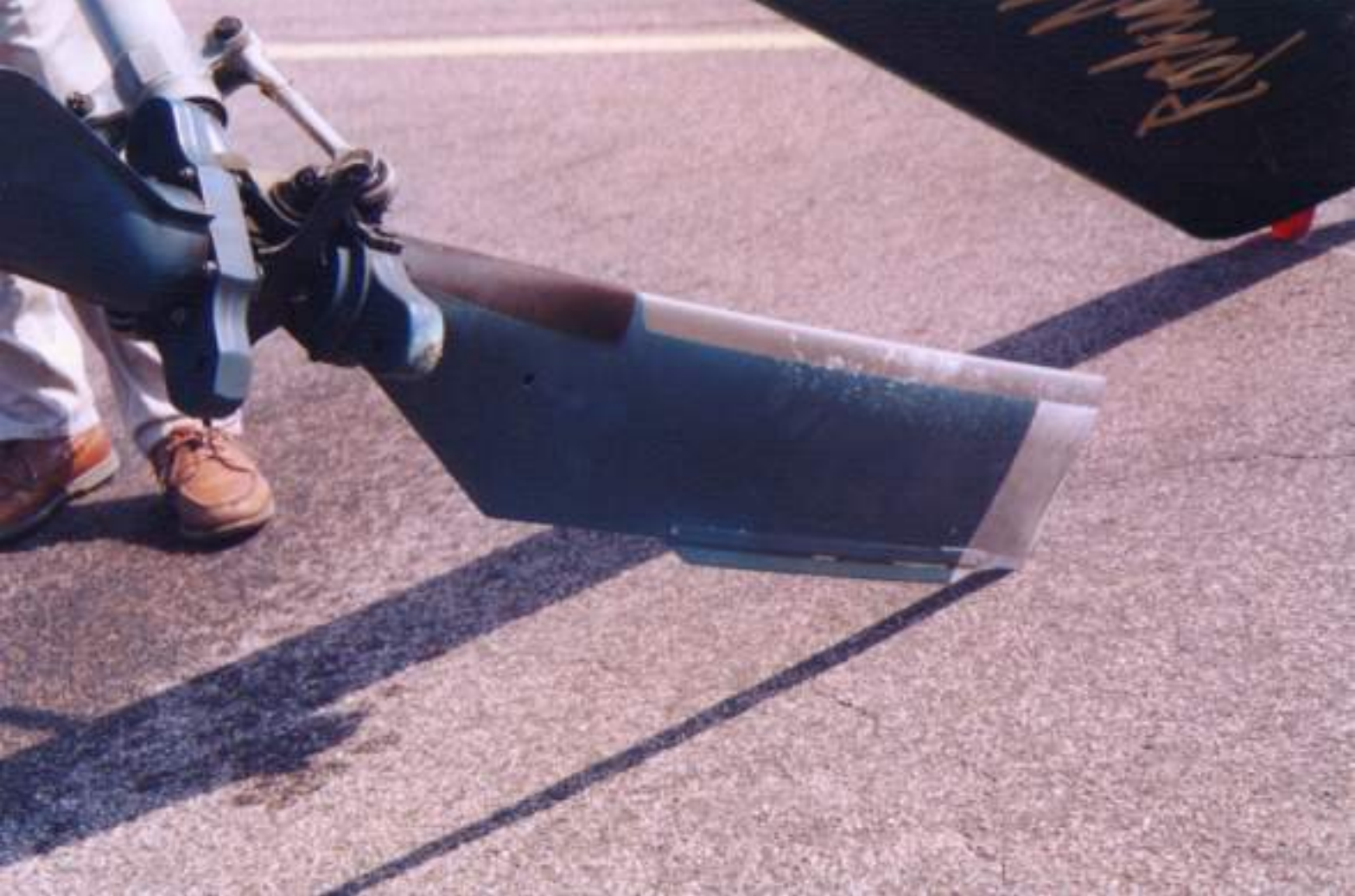
Photo 21. Tail Rotor Blade With Leading Edge Scaring
