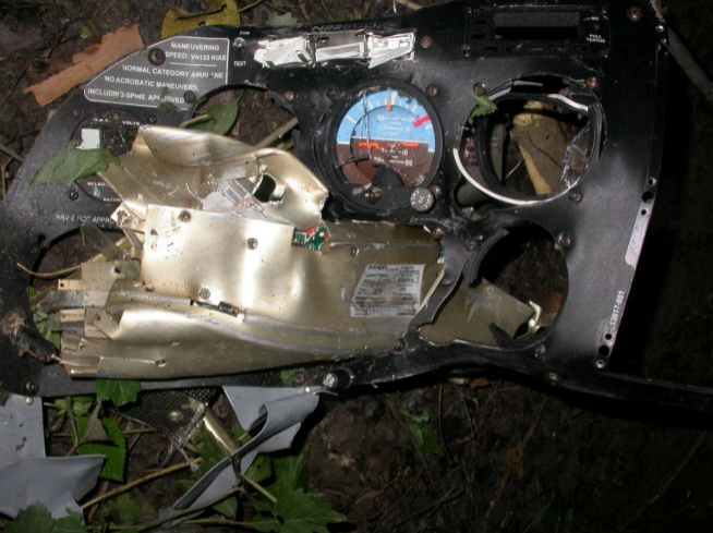
Photo 20. View of the instrument panel with the attitude gyro still attached.
