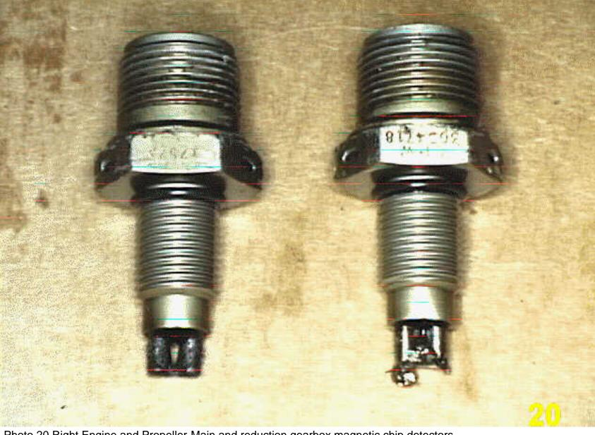
Photo 20 Right Engine and Propeller-Main and reduction gearbox magnetic chip detectors
