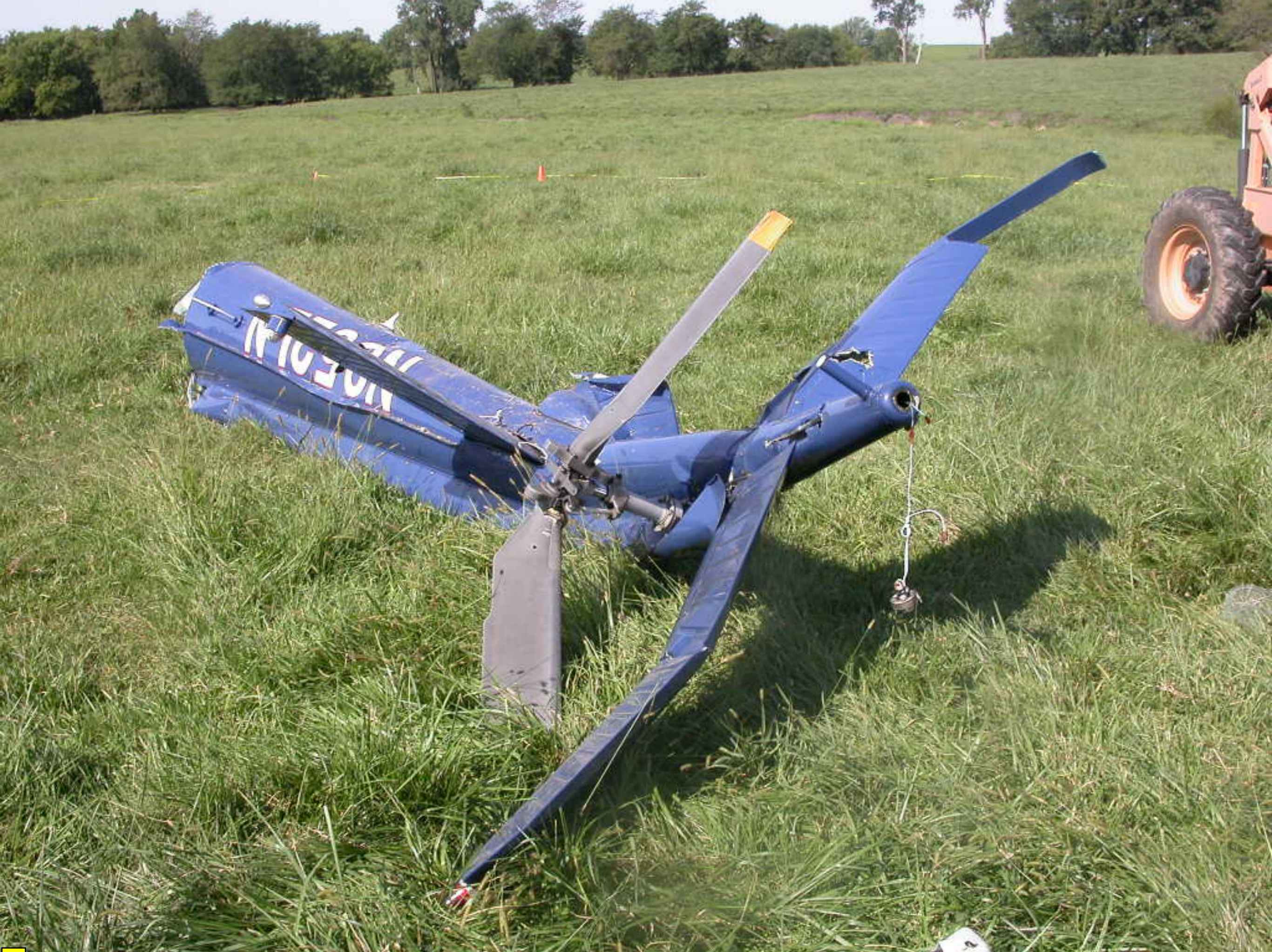
Photo 20: View of tail boom, tail rotor, and empennage removed from the main wreckage
