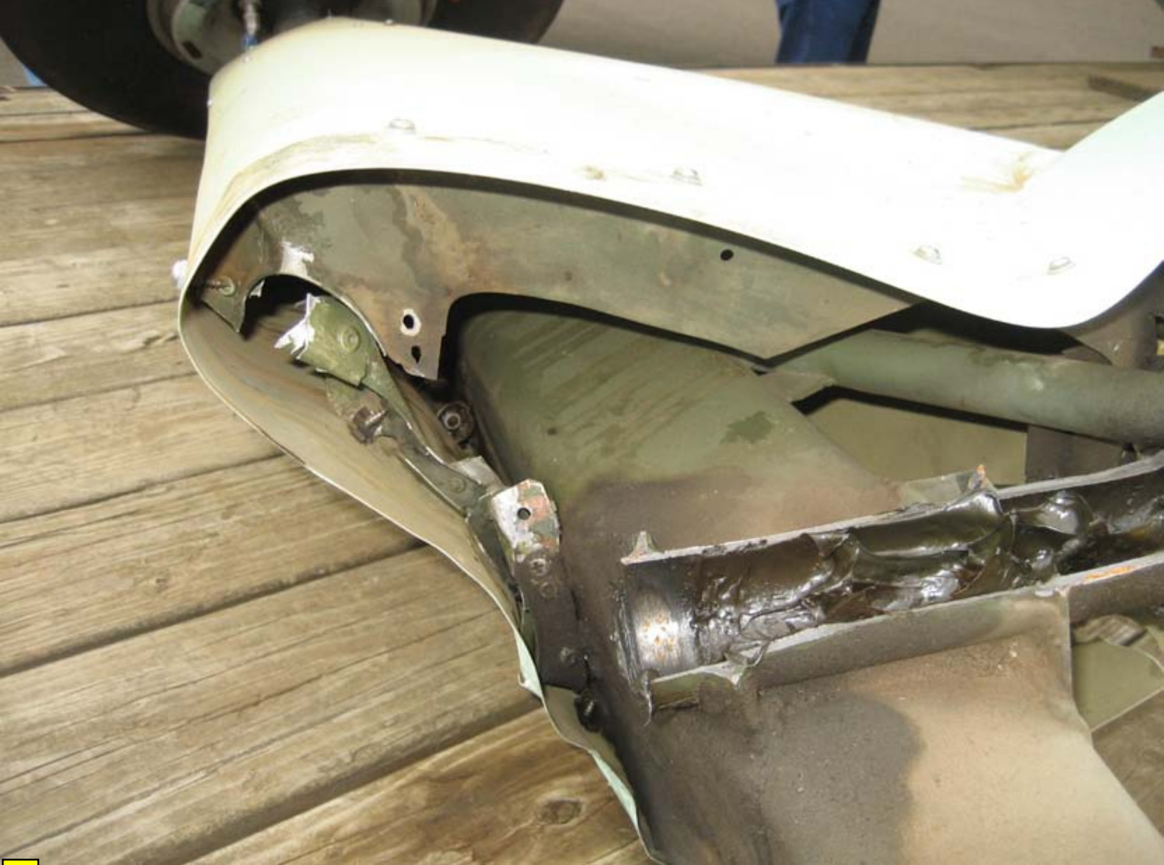
Photo 2. Landing gear structure failure
