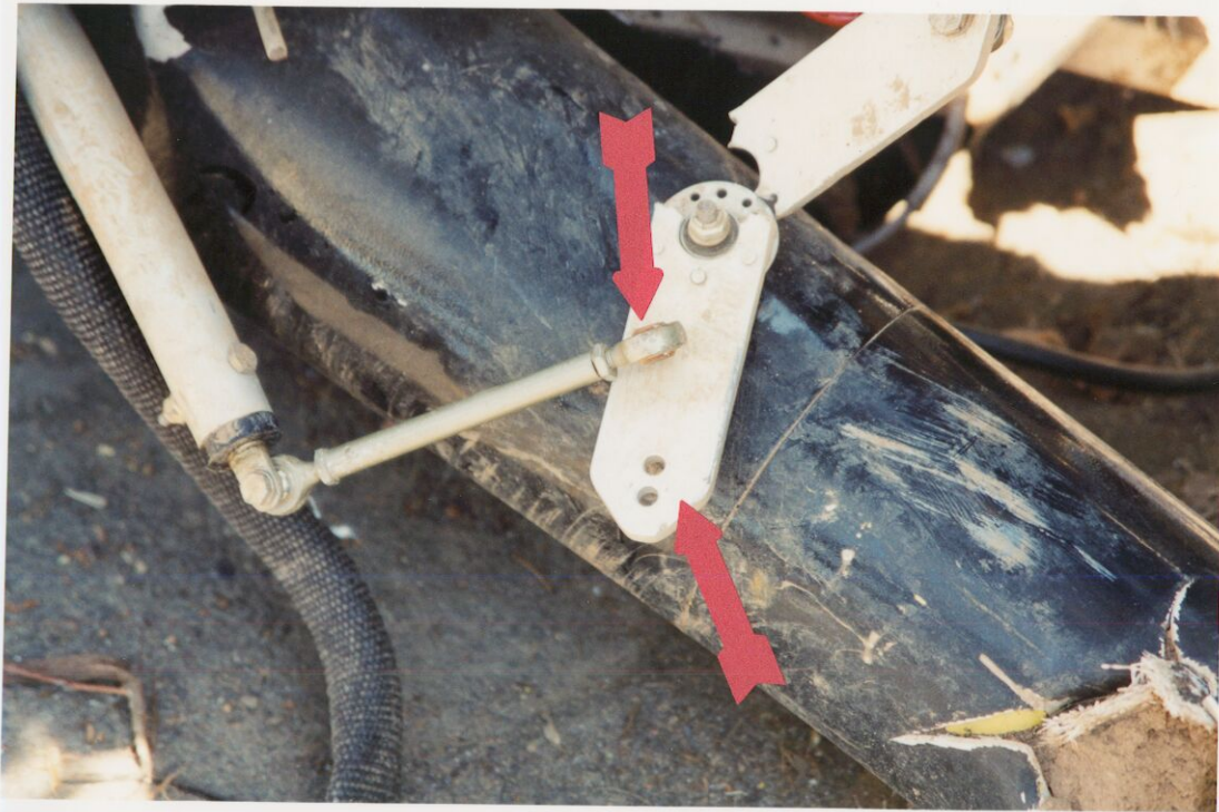
Photo 2. Bell crank and associated linkage.
