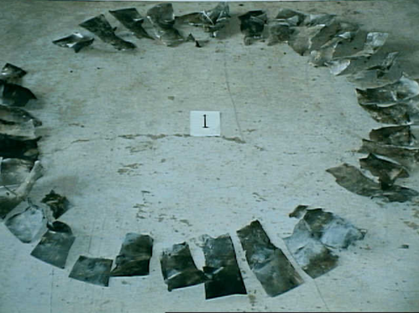
Photo 2. No. 1 engine fan blade fragments
