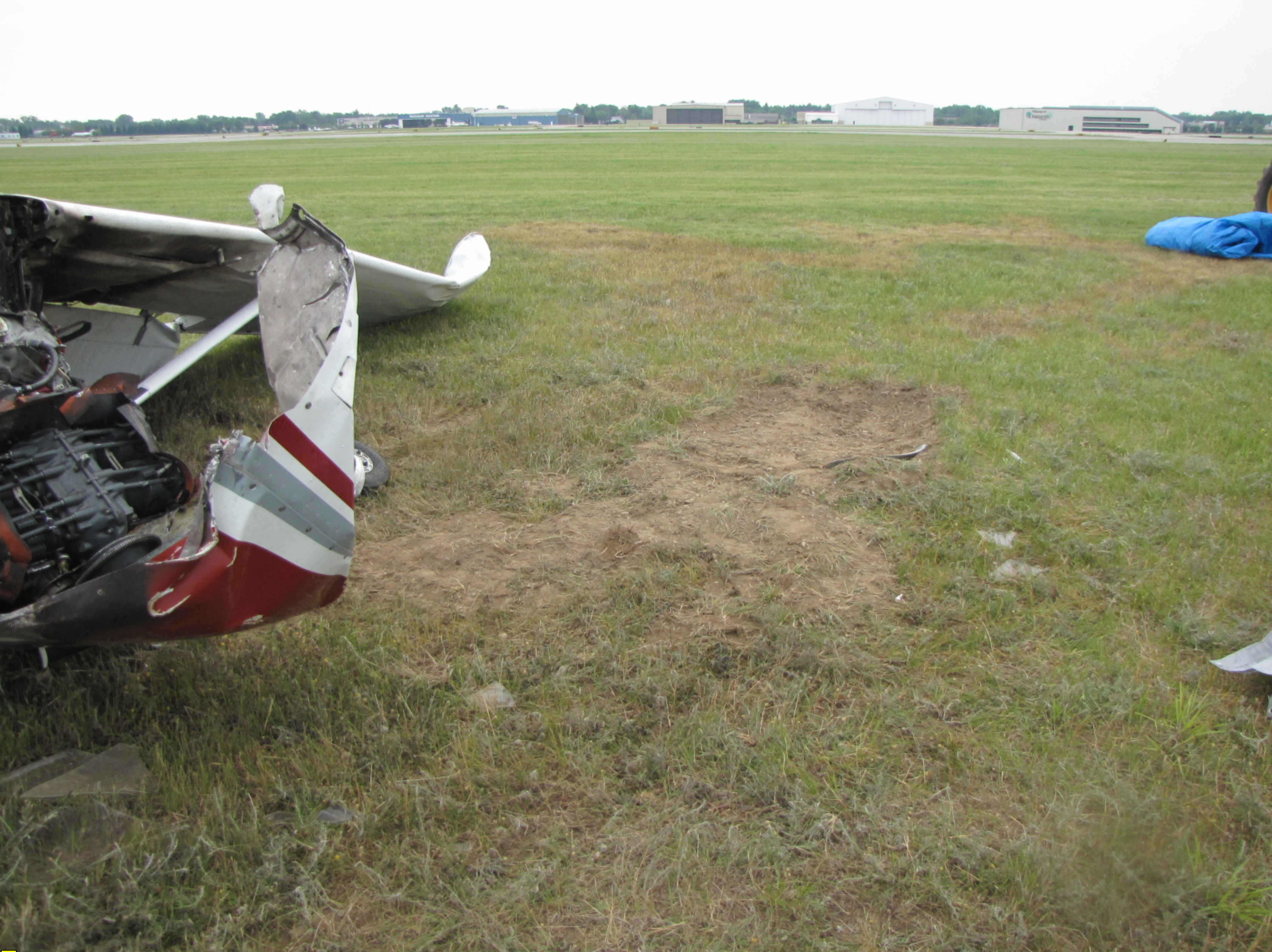
Photo 2 - Ground scar and fuel stains.
