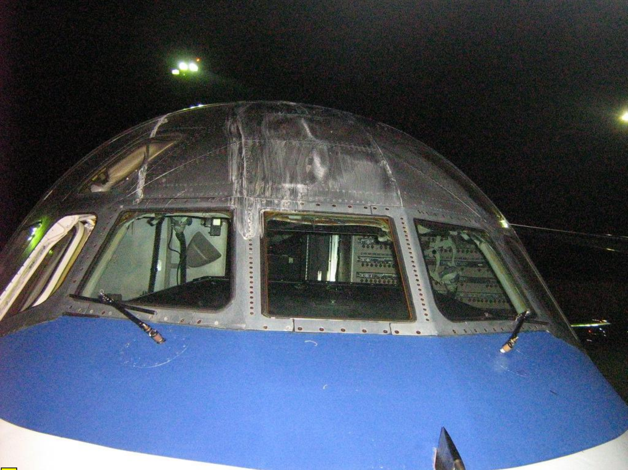
Photo 2 - Cockpit damage to N70504, McDonnell Douglas DC-9-82
