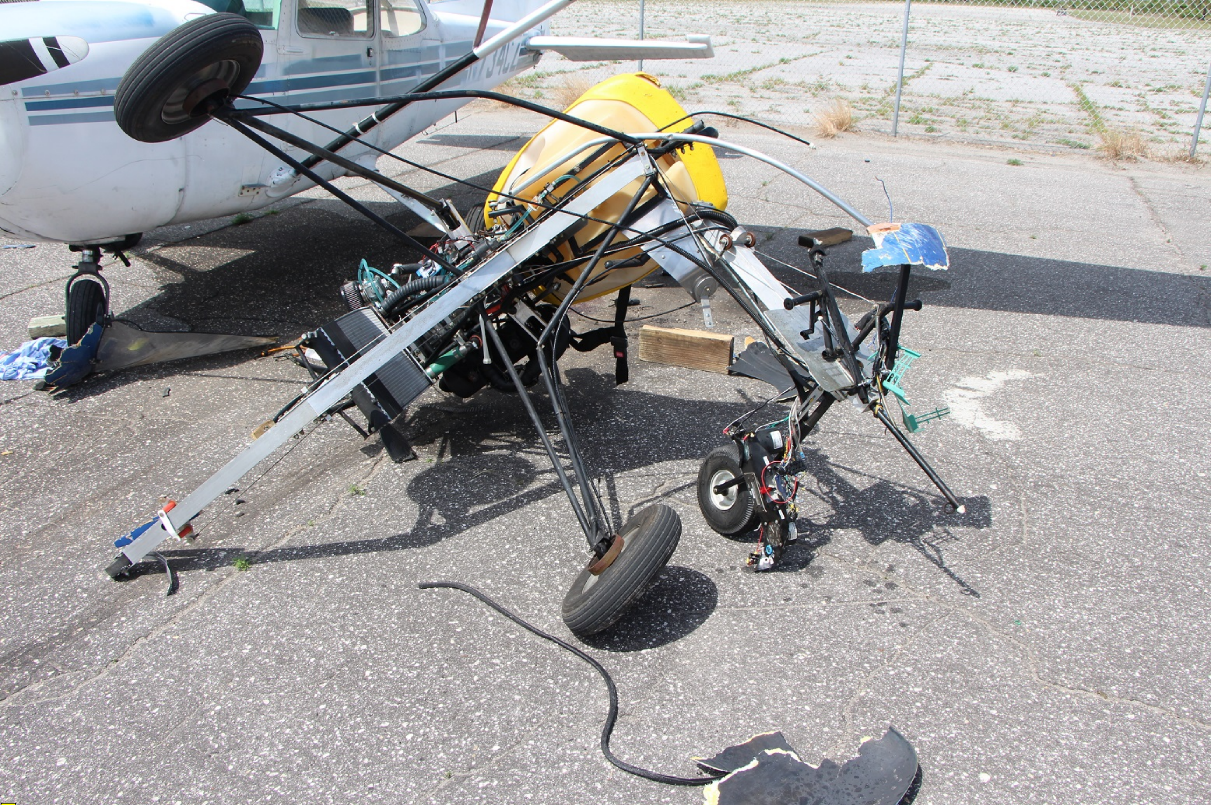
Photo 6: Bent Gear, Fractured Keel, and Undamaged Pitot Tube.
