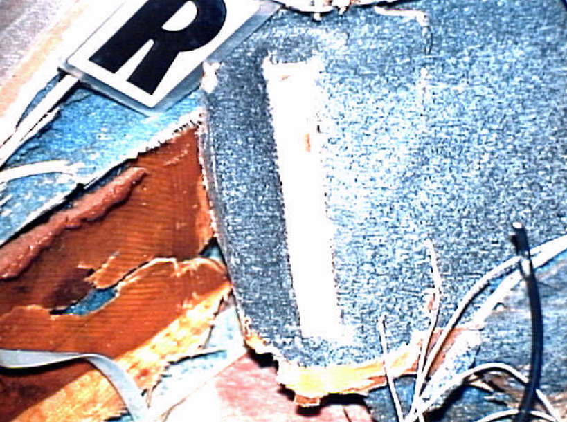
Photo 19. Right rear fuel sight gauge.
