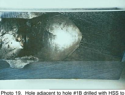
Photo 19. Hole adjacent to hole #1B drilled with HSS to failure by increased cutting data and without coolant. BEA has been performed.
