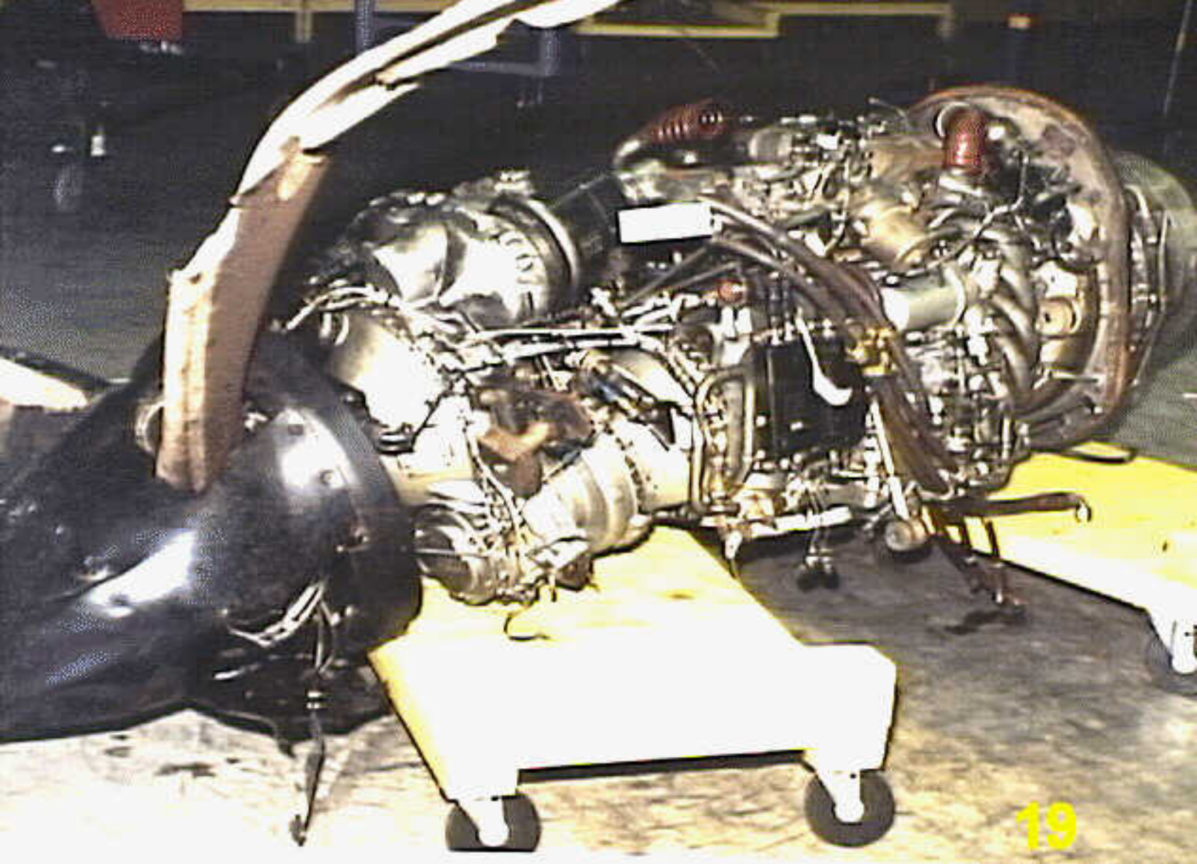
Photo 19 Right Engine and Propeller-The turbomachine, reduction gearbox and propeller
