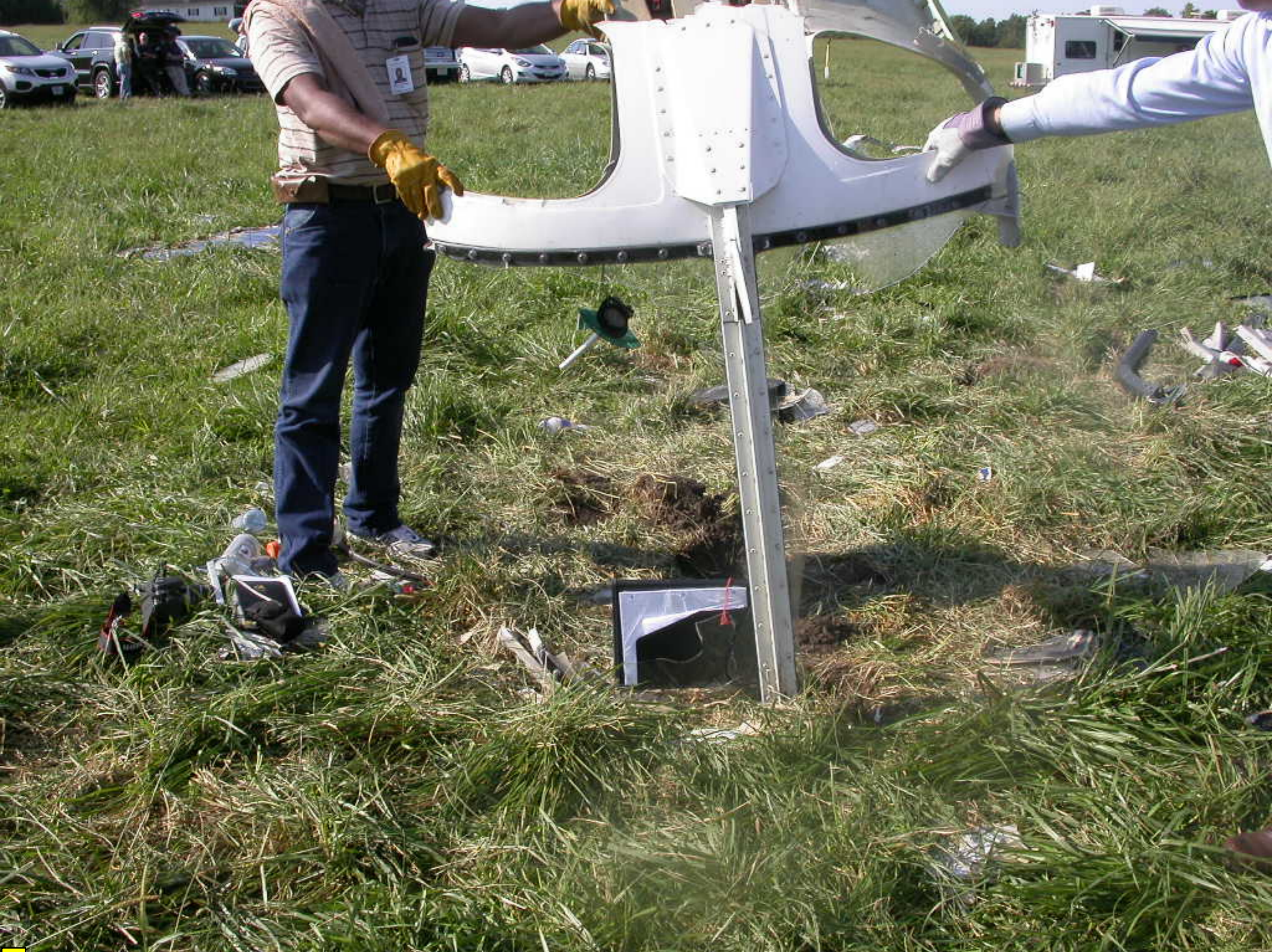
Photo 19: Windshield frame at the initial impact point
