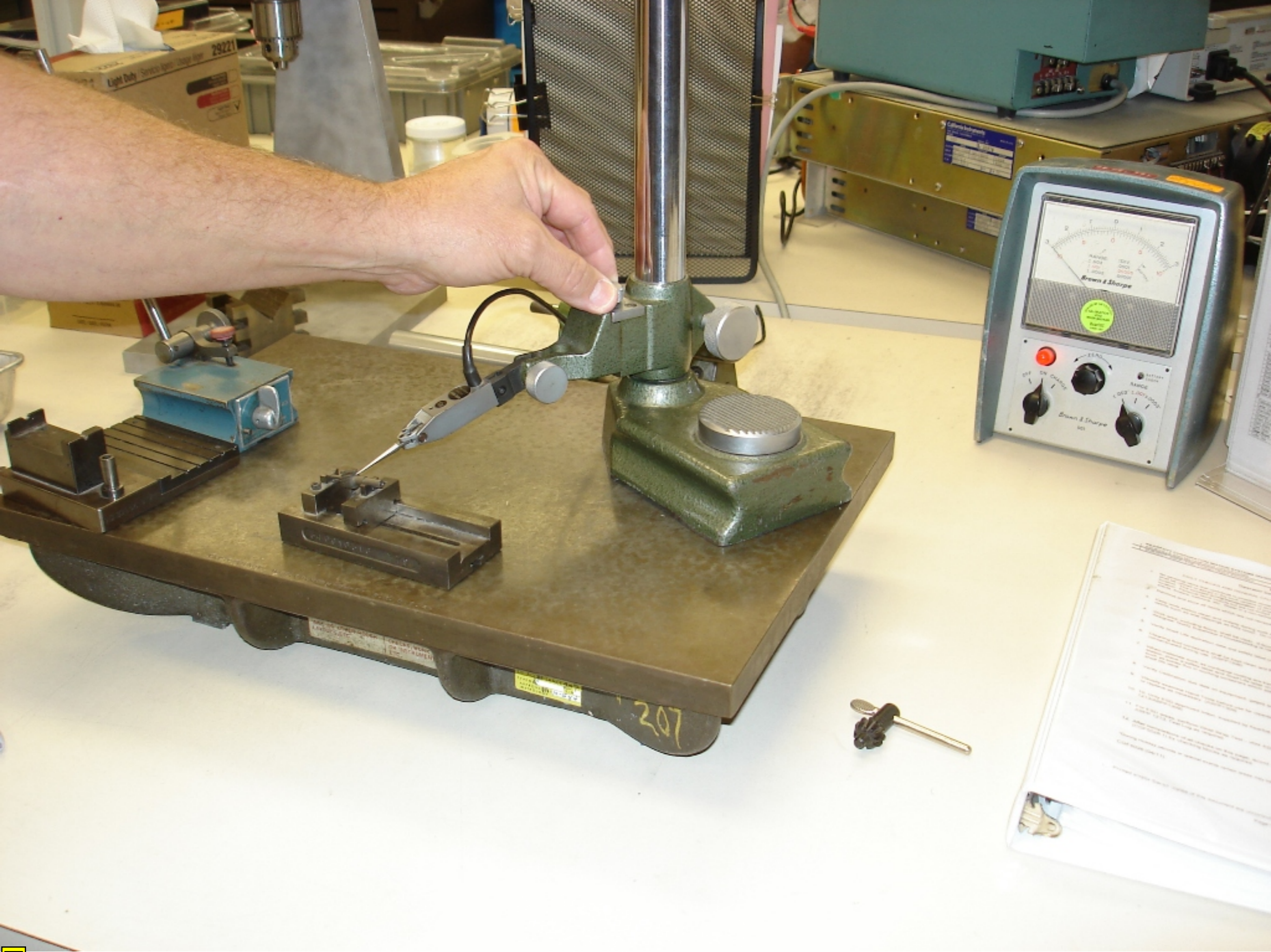
Photo 18. Measuring the bend in the output shaft.
