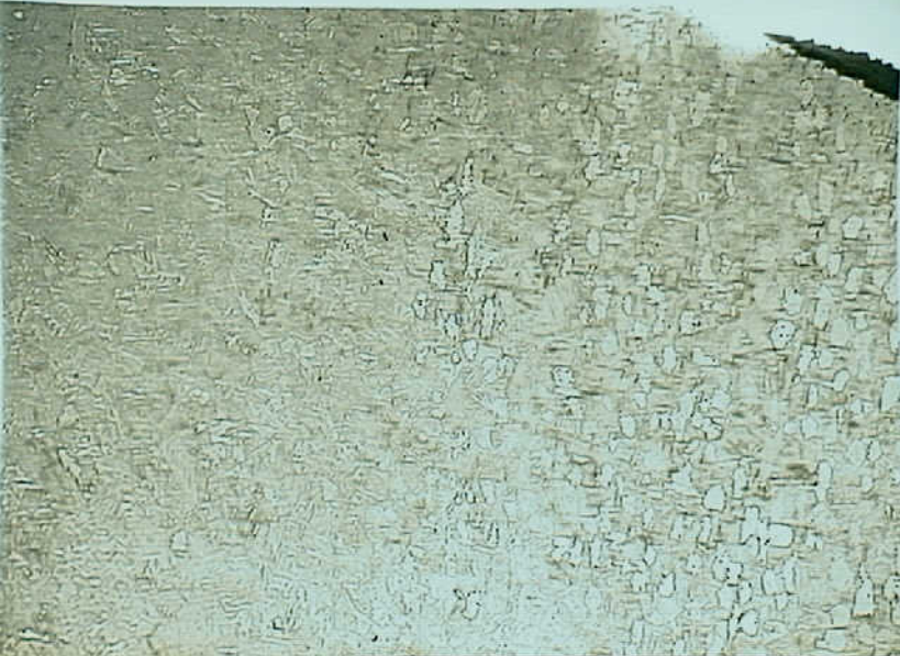
Photo 18. Hole #1A. Longitudinal section of showing overheated material (above B-transus) with transformed B and partially transformed B. The section is located at arrow B in photo 16. Mag 200X
