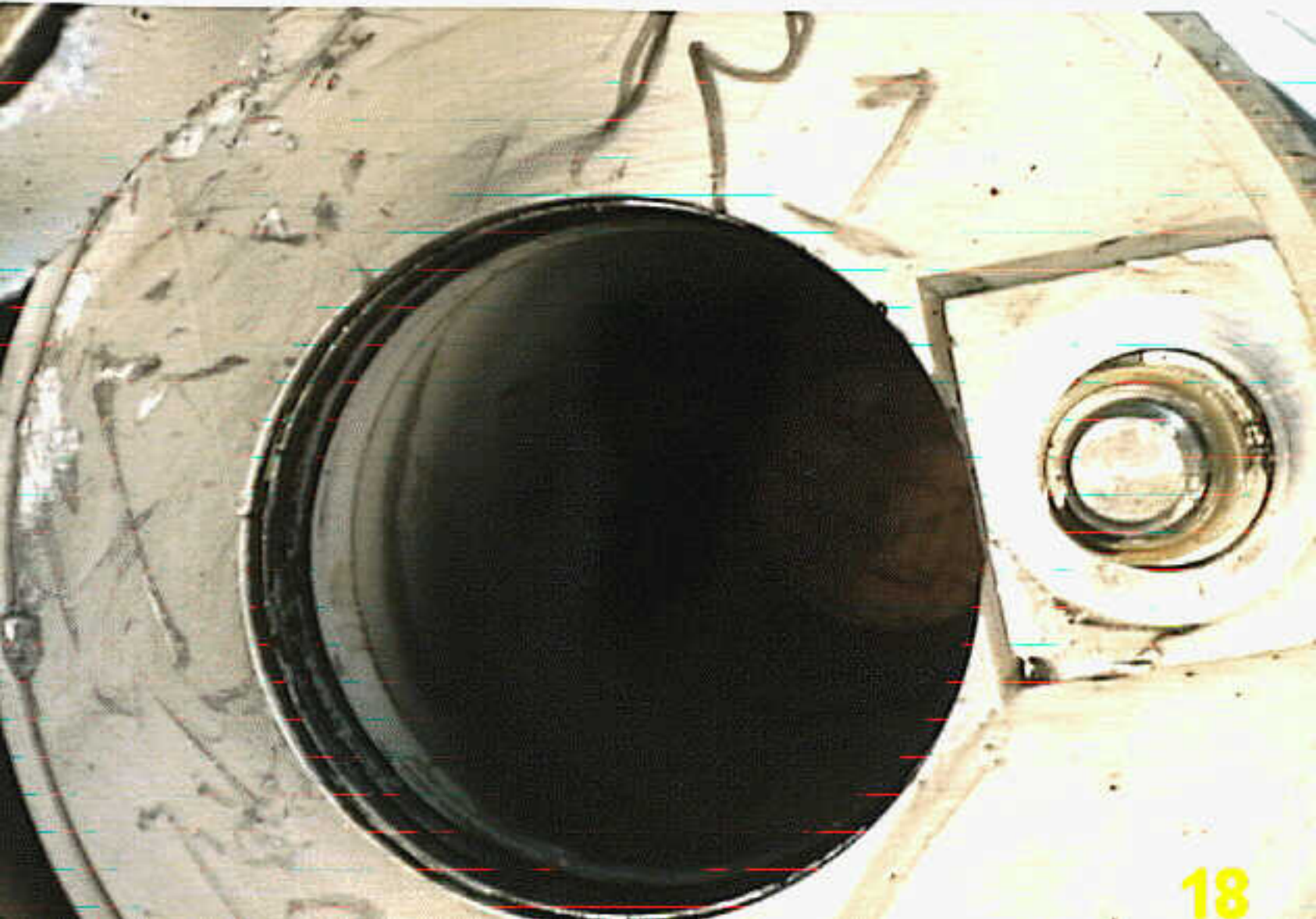
Photo 18 Right Engine and Propeller-No.1 propeller blade taper bore and pitch change pin
