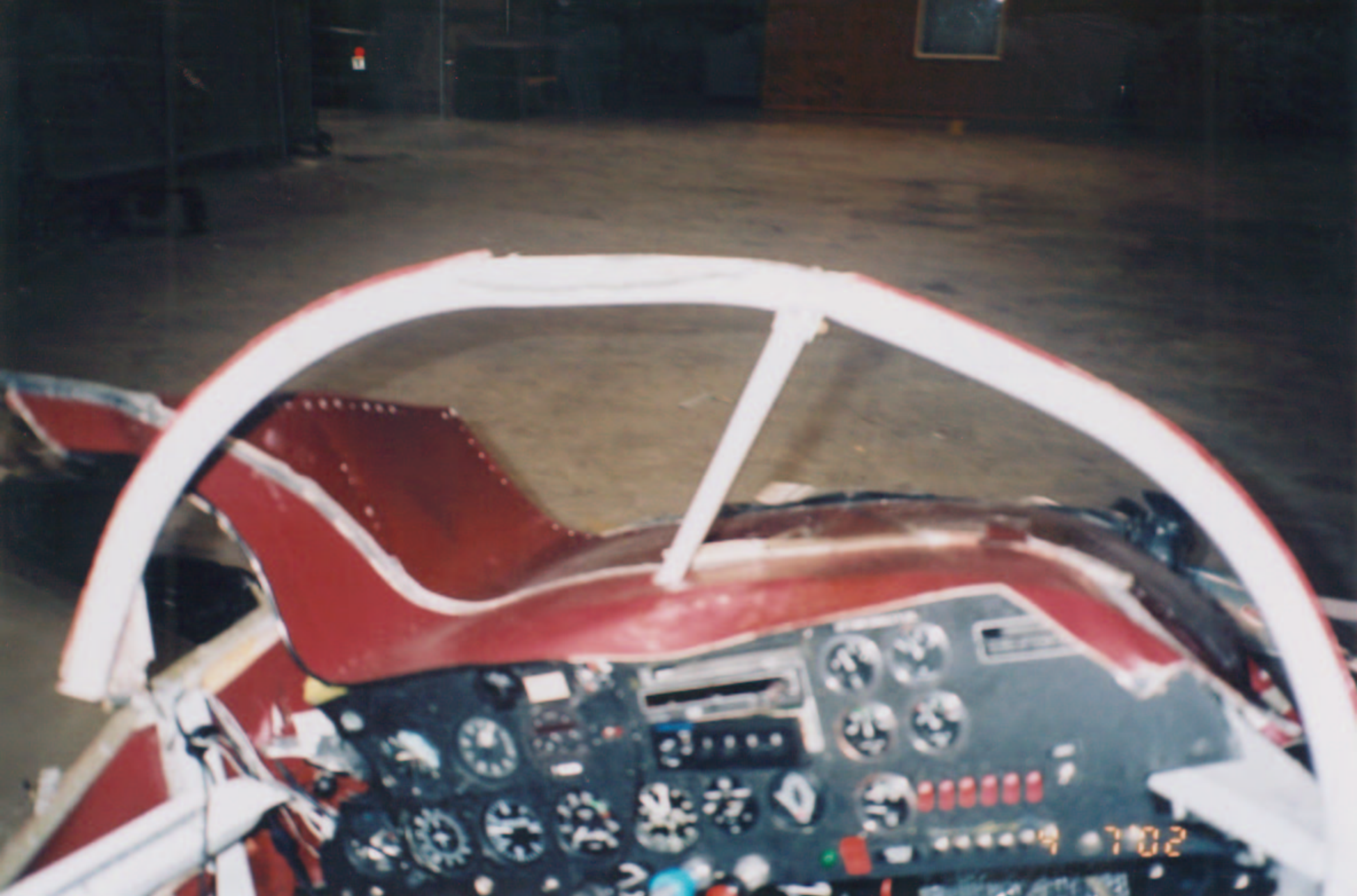
Photo 18 - Photo of N3333S upper windshield support brace
