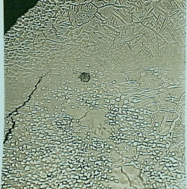
Photo 17. Hole #1A. Longitudinal section showing remelt material with cracks and overheated material (above B-transus) with transformed B. The section is located at arrow A in photo 16. Mag 500X.
