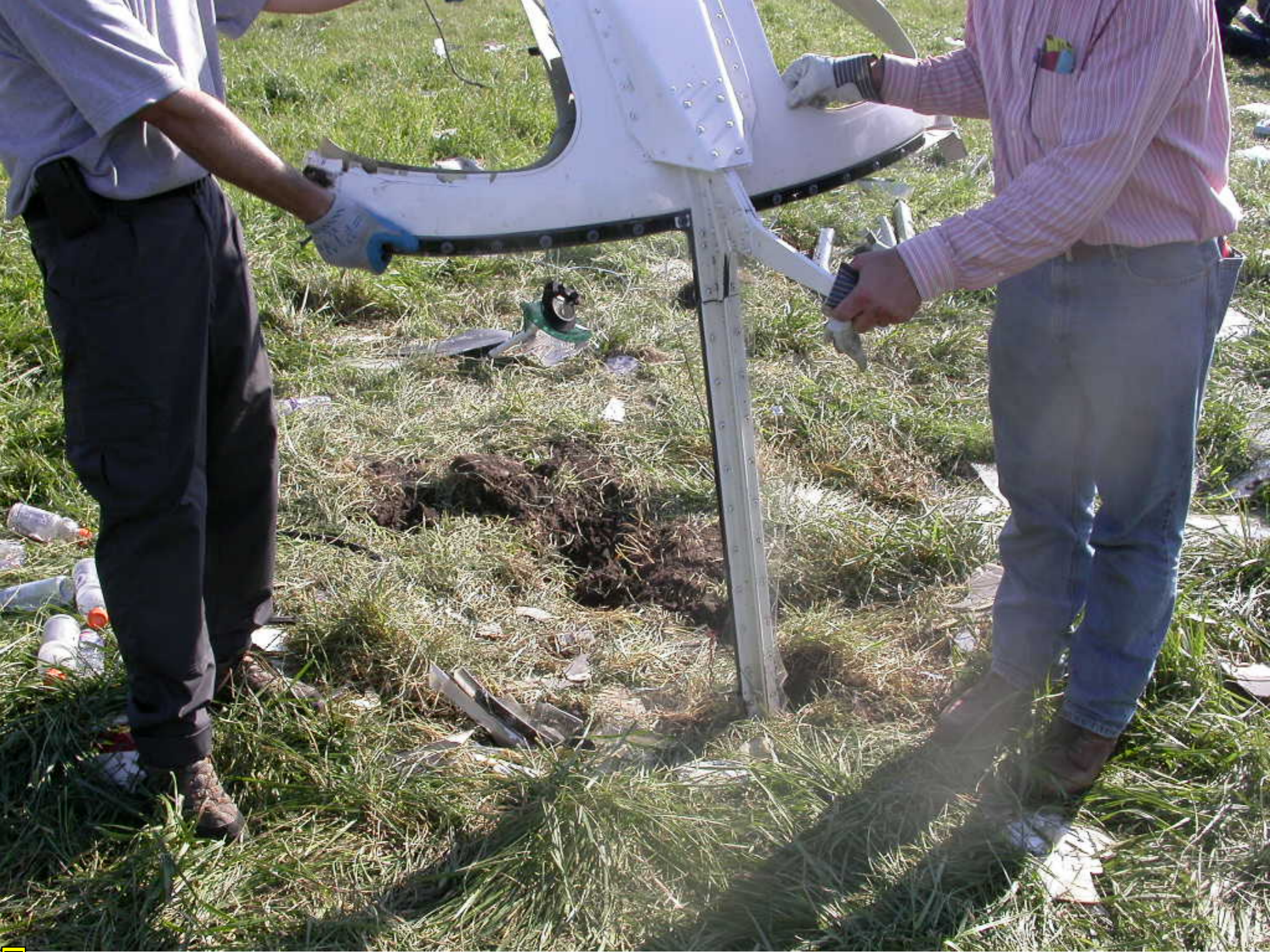
Photo 17: View of the windshield frame oriented over the initial point of impact
