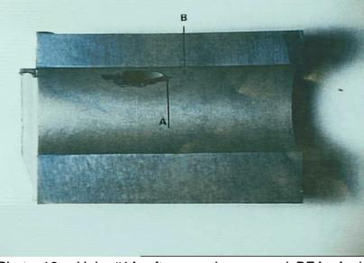
Photo 16. Hole #1A after opening up and BEA. And elliptic cavity can be seen on the ID. The surrounding area of the cavity indicated alternaterly in grey and blue.
